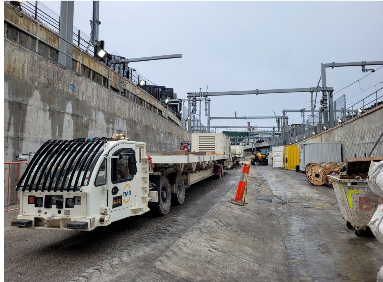
Multi Service Vehicle (MSV) transports material into the tunnels
