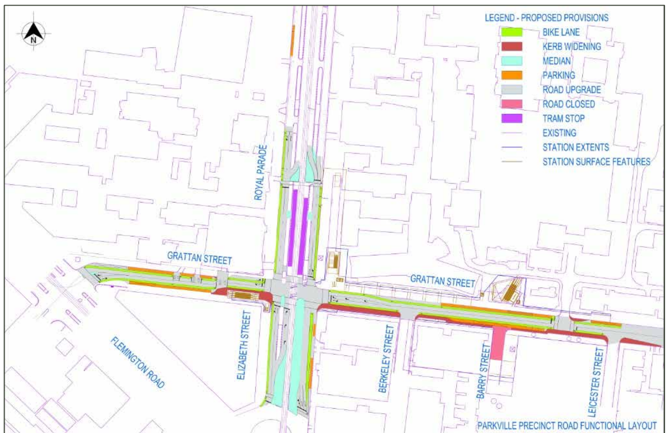
Figure 9-6 Parkville station precinct road functional layout
