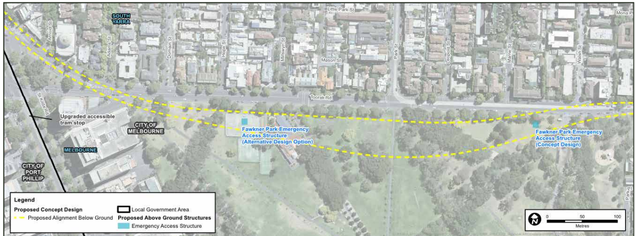
Figure 7-3 Fawkner Park Melbourne Metro legacy emergency access structures
