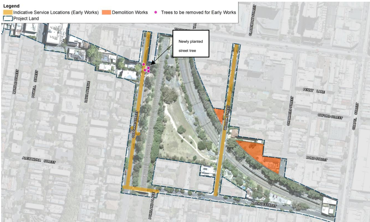
Figure 12. Excerpt from the Site Layout Plan which identifies Early Works within the Eastern Portal (refer to Appendix 1).
