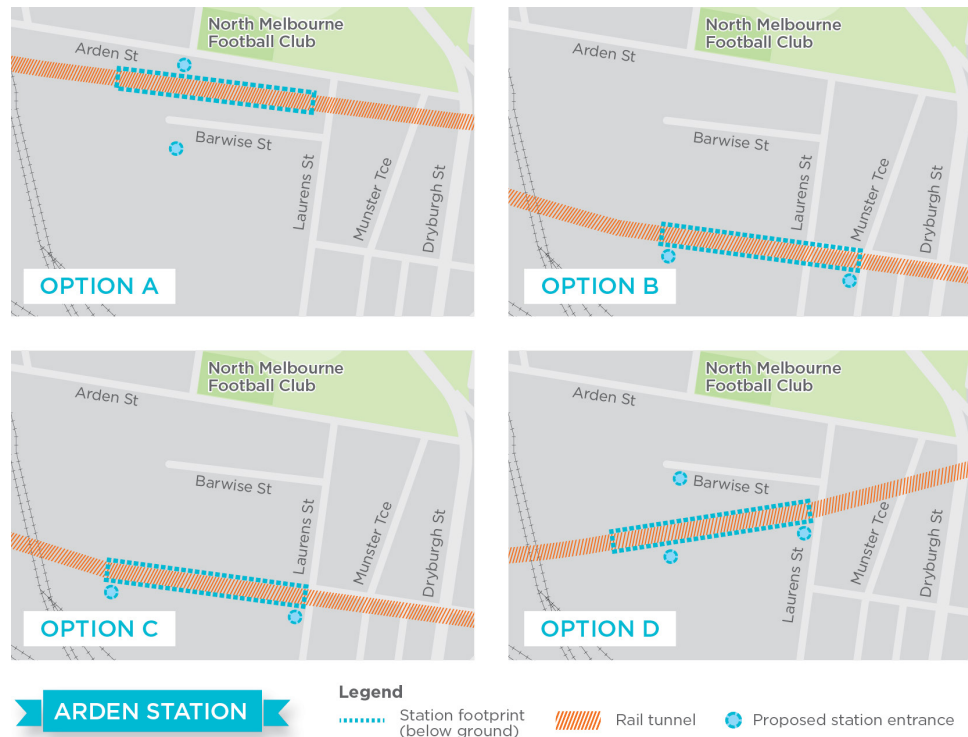
Figure 5-9 Potential Arden station positions
