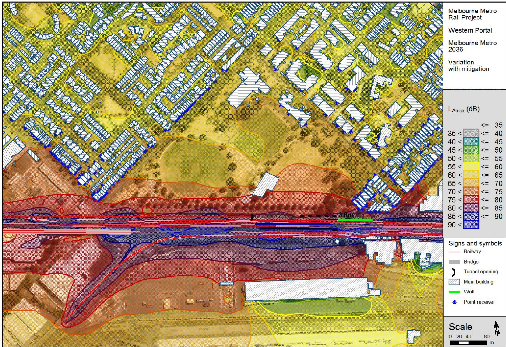
Figure C.27: Western Portal with Melbourne Metro Concept Design (with Mitigation), L_{Amax} predicted noise levels. Barrier height is above the rail height for the RRL and Newport group of trains
