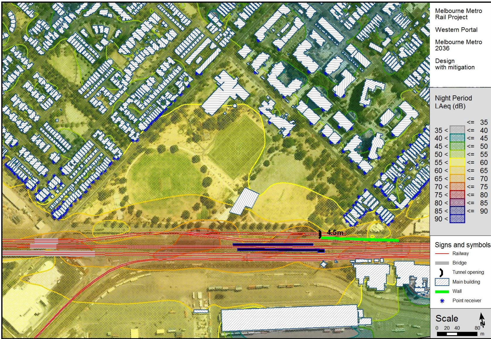
Figure C23: Western Portal with Melbourne Metro Concept Design (with Mitigation), Night Period predicted noise levels. Barrier height is above the rail height for the RRL and Newport group of trains
