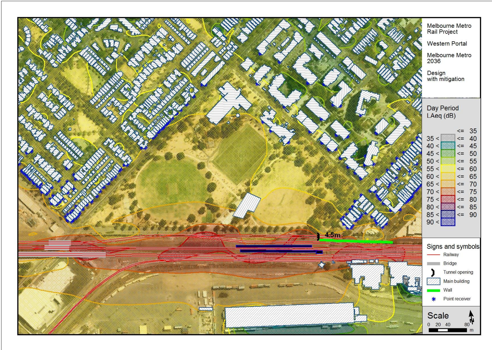
Figure C.22: Western Portal with Melbourne Metro Concept Design (with Mitigation), Day Period predicted noise levels. Barrier height is above the rail height for the RRL and Newport group of trains
