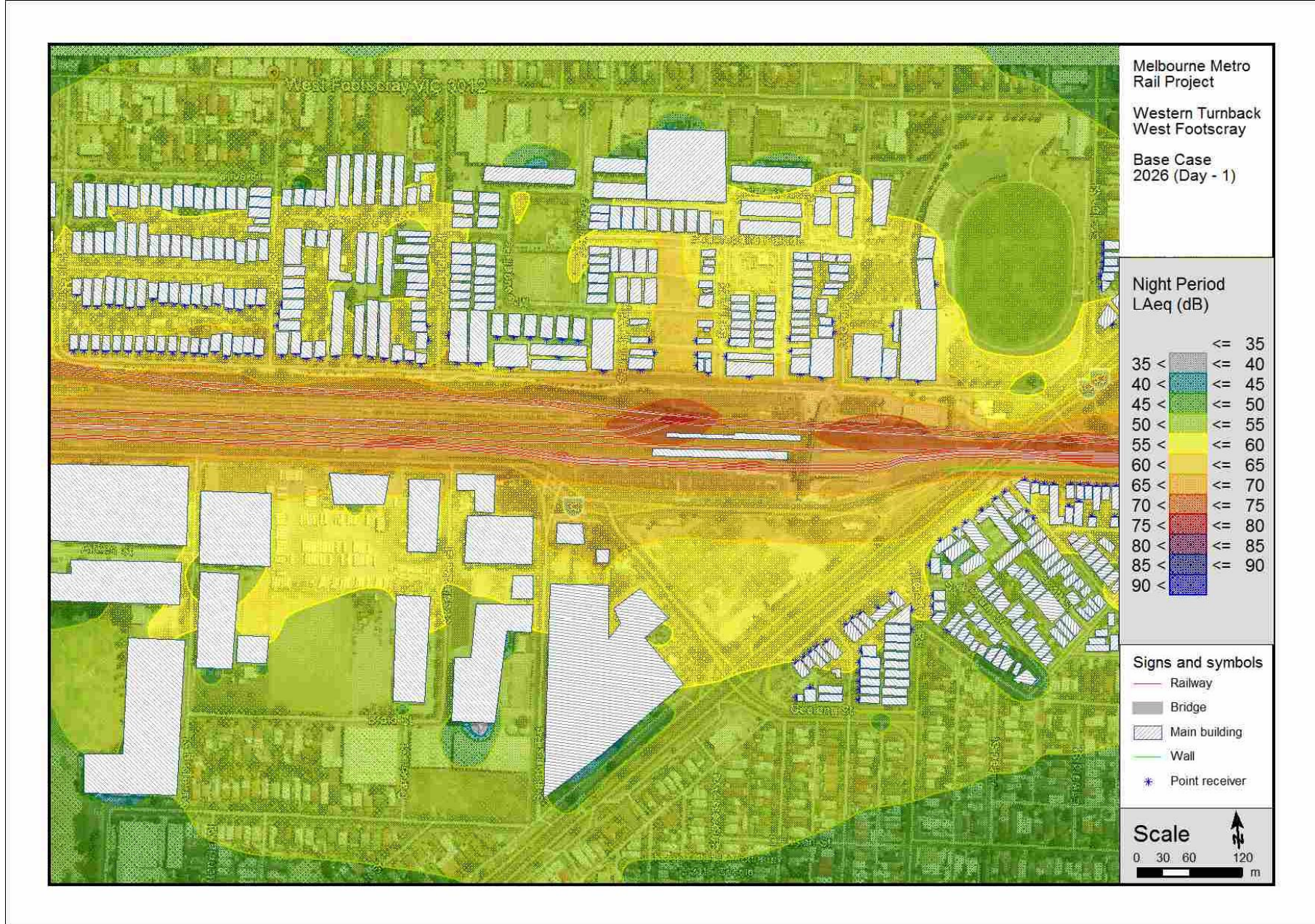
Figure C.17: Western Turnback at West Footscray Base-Case 2026, Night Period, predicted train noise levels
