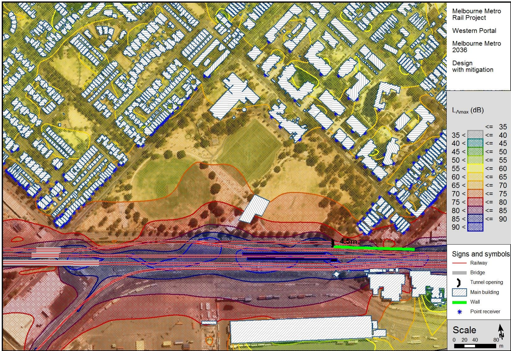
Figure C.24: Western Portal with Melbourne Metro Concept Design (with Mitigation), L_{Amax} predicted noise levels. Barrier height is above the rail height for the RRL and Newport group of trains
