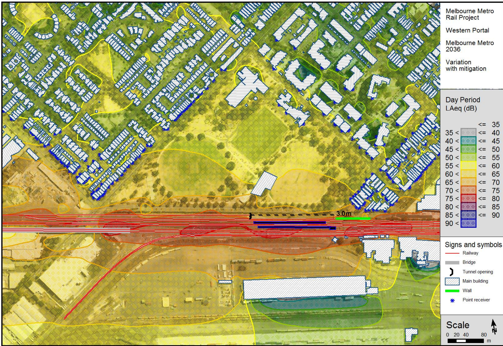
Figure C.25: Western Portal with Melbourne Metro Concept Design (with Mitigation), Day Period predicted noise levels. Barrier height is above the rail height for the RRL and Newport group of trains
