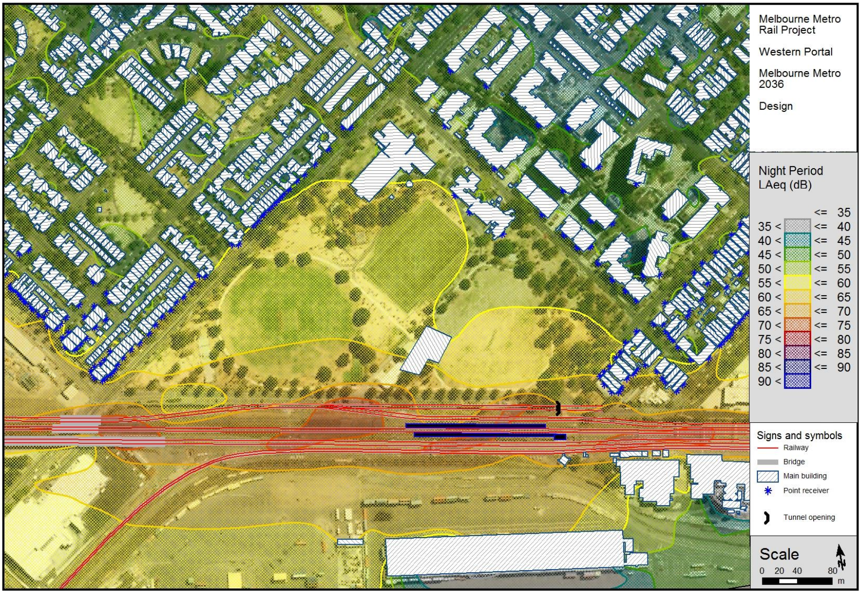
Figure C.5: Western Portal Melbourne Metro Concept Design 2036, Night Period, predicted train noise levels
