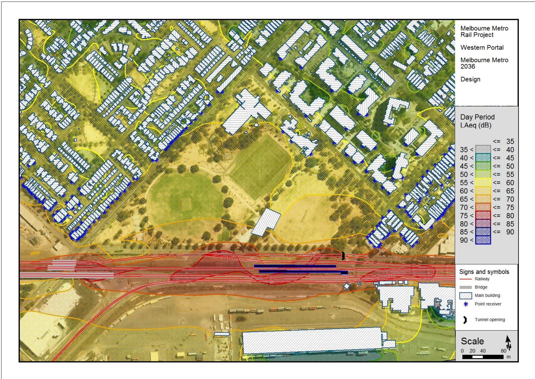
Figure C.4: Western Portal Melbourne Metro Concept Design 2036, Day Period, predicted train noise levels
