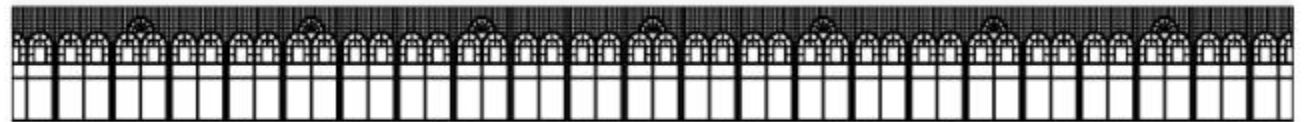
PANELS ACTUAL LAYOUT ON SITE 27M LONG (END PANELS CUT ON SITE)
