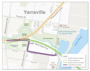
Designed for the long tunnel, this option includes ramps that run either side of the existing freeway.
