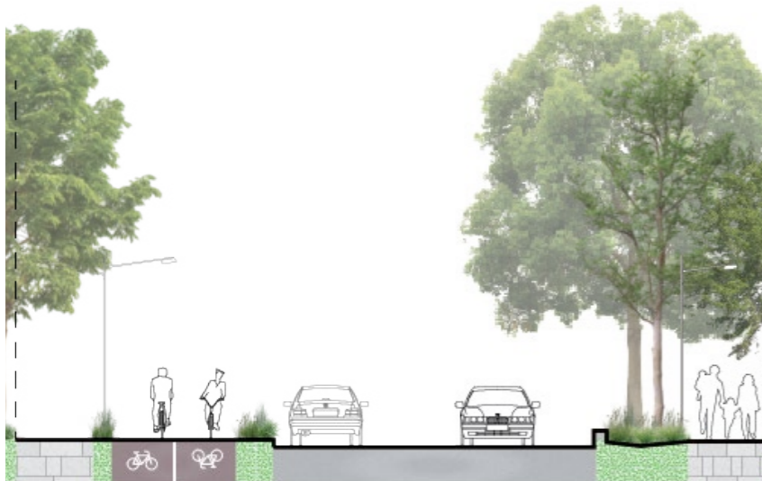
Indicative Section, Green Street Section- Type C - Cycling
