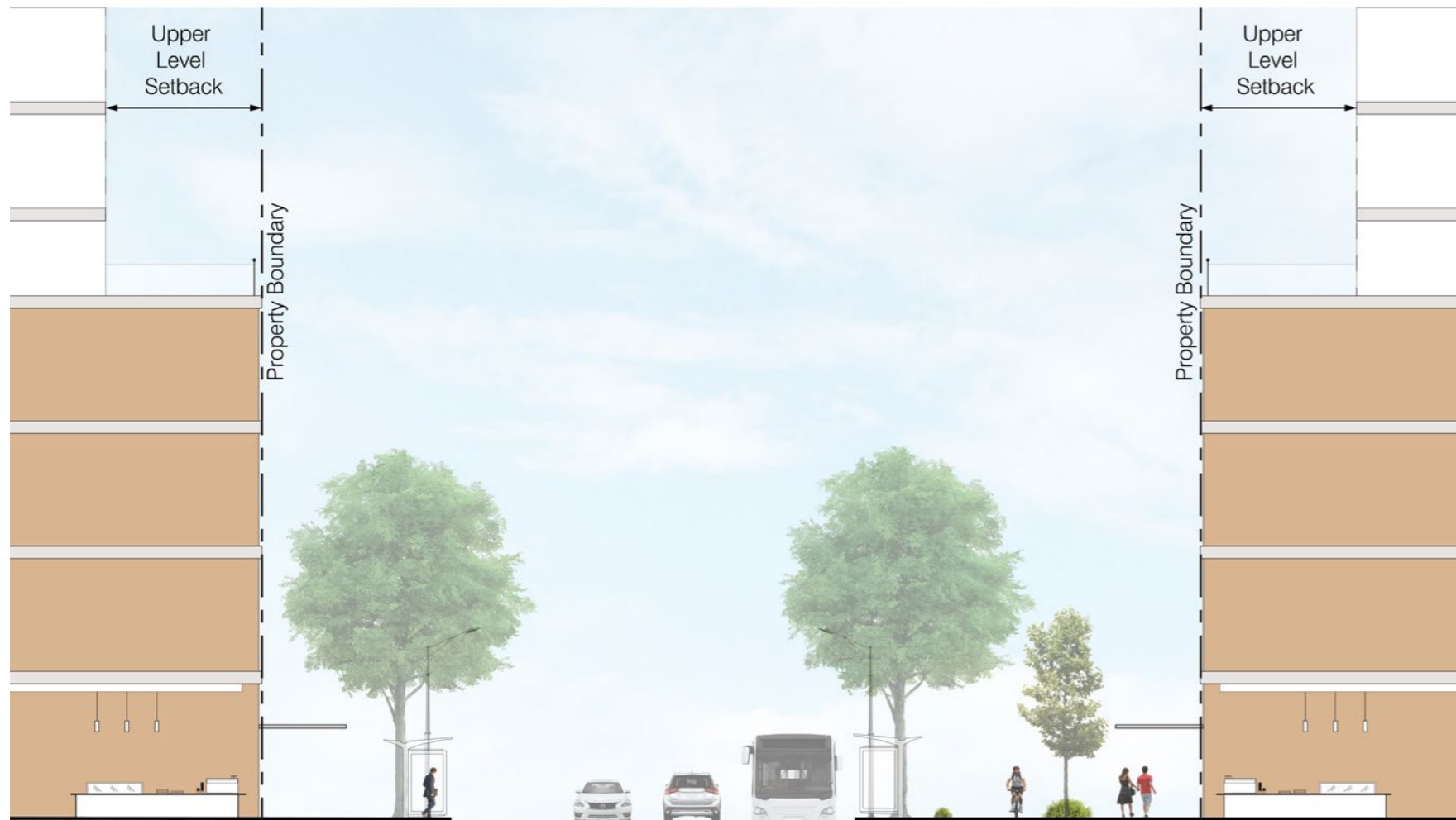
Figure 6.8: Potential section - Activity Street
