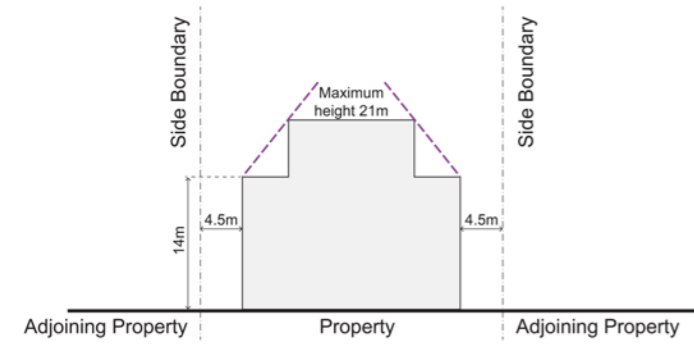
Figure 6.46: Garden Apartment section sides
