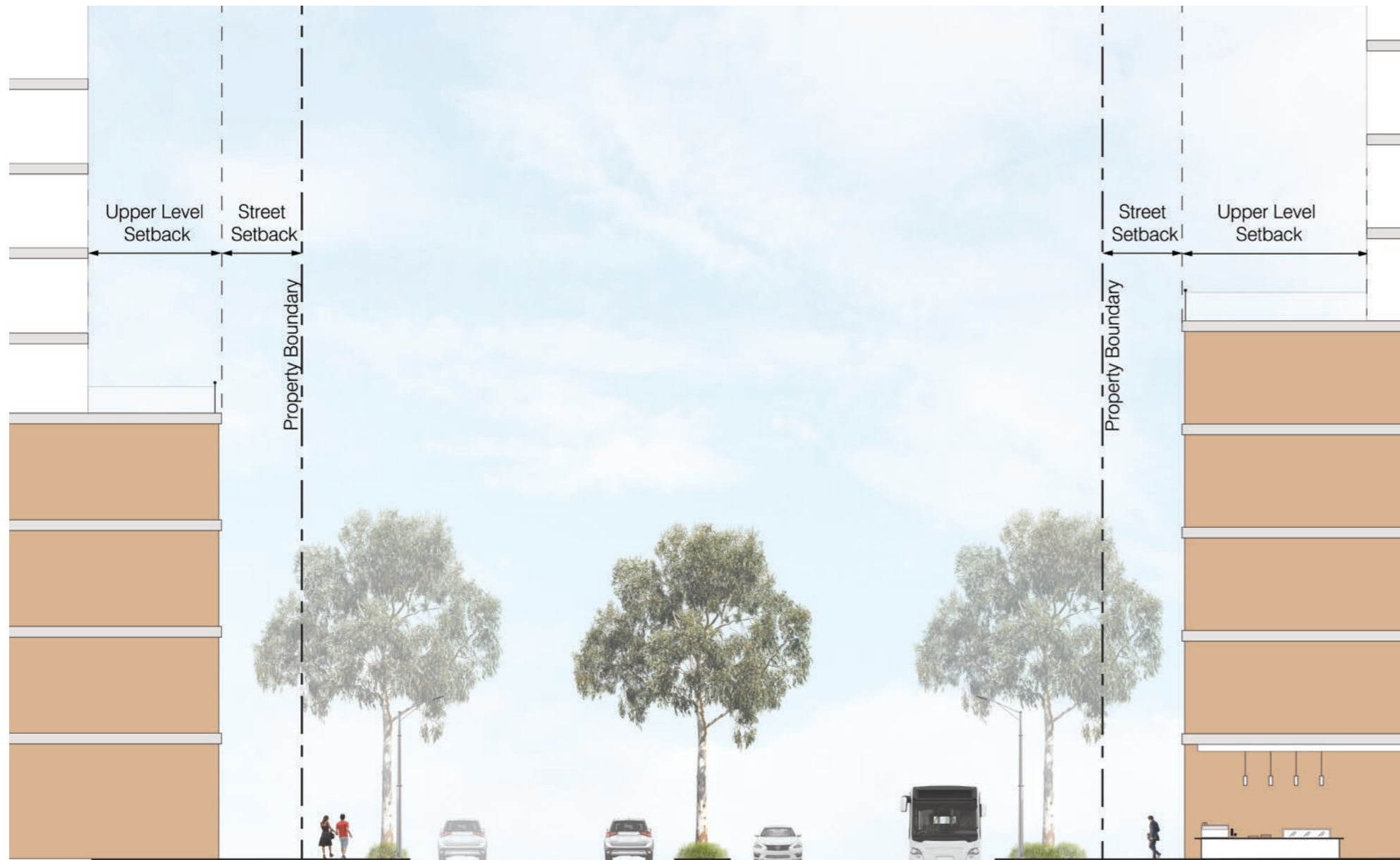
Figure 6.23: Potential section - Avenue
