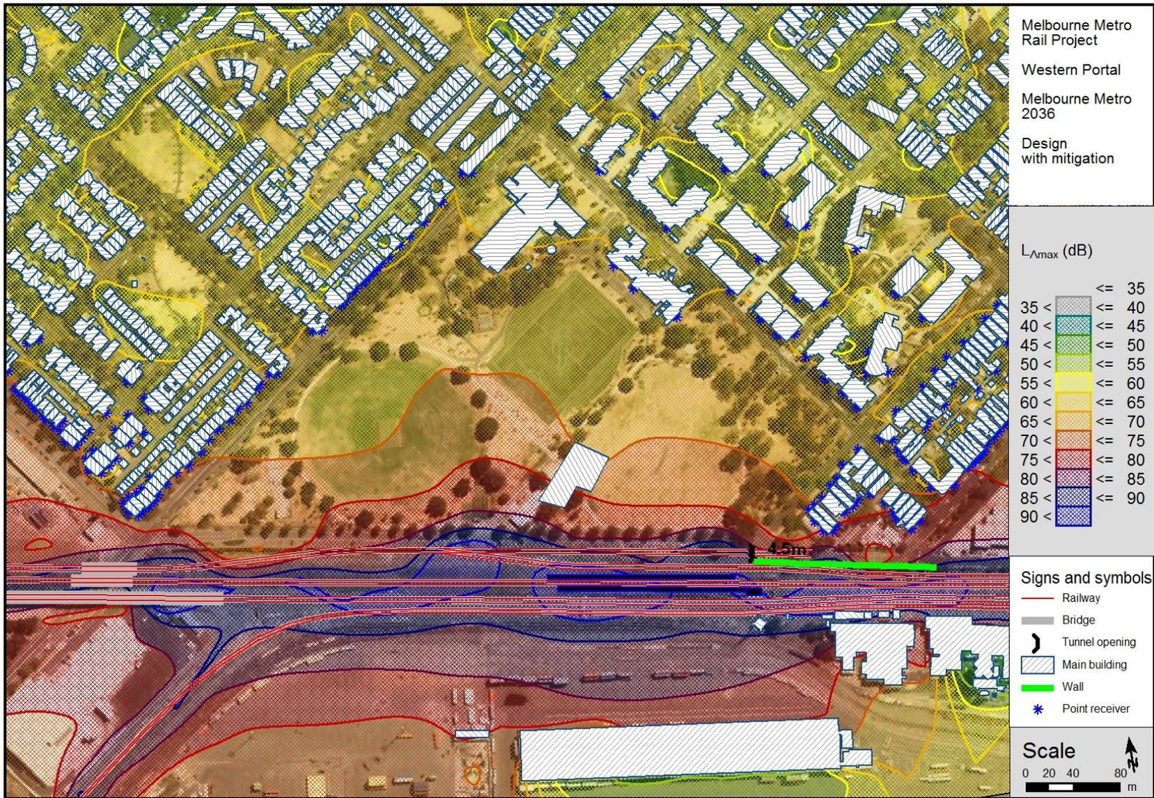
Figure C.24: Western Portal with Melbourne Metro Concept Design (with Mitigation),  $L_{Amax}$  predicted noise levels. Barrier height is above the rail height for the RRL and Newport group of trains
