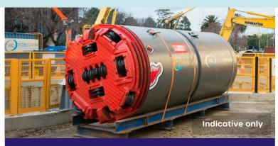
Three mini tunnel boring machines (TBMs) will dig under Bulleen to build the new Yarra East Main Sewer (YEMS). The TBMs will work together to dig the new sewer.
