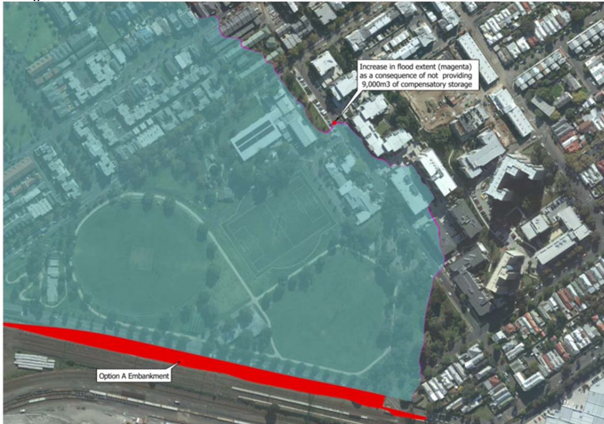
Figure 8 - Increase in Flood Extent as a Consequence of not Providing Compensatory Storage (9,000 m 3 )
