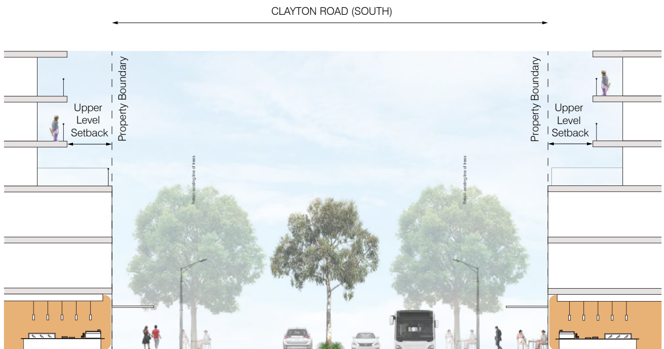
Figure 25: Section A - Illustration of potential typical section of Clayton Road south of the rail line
