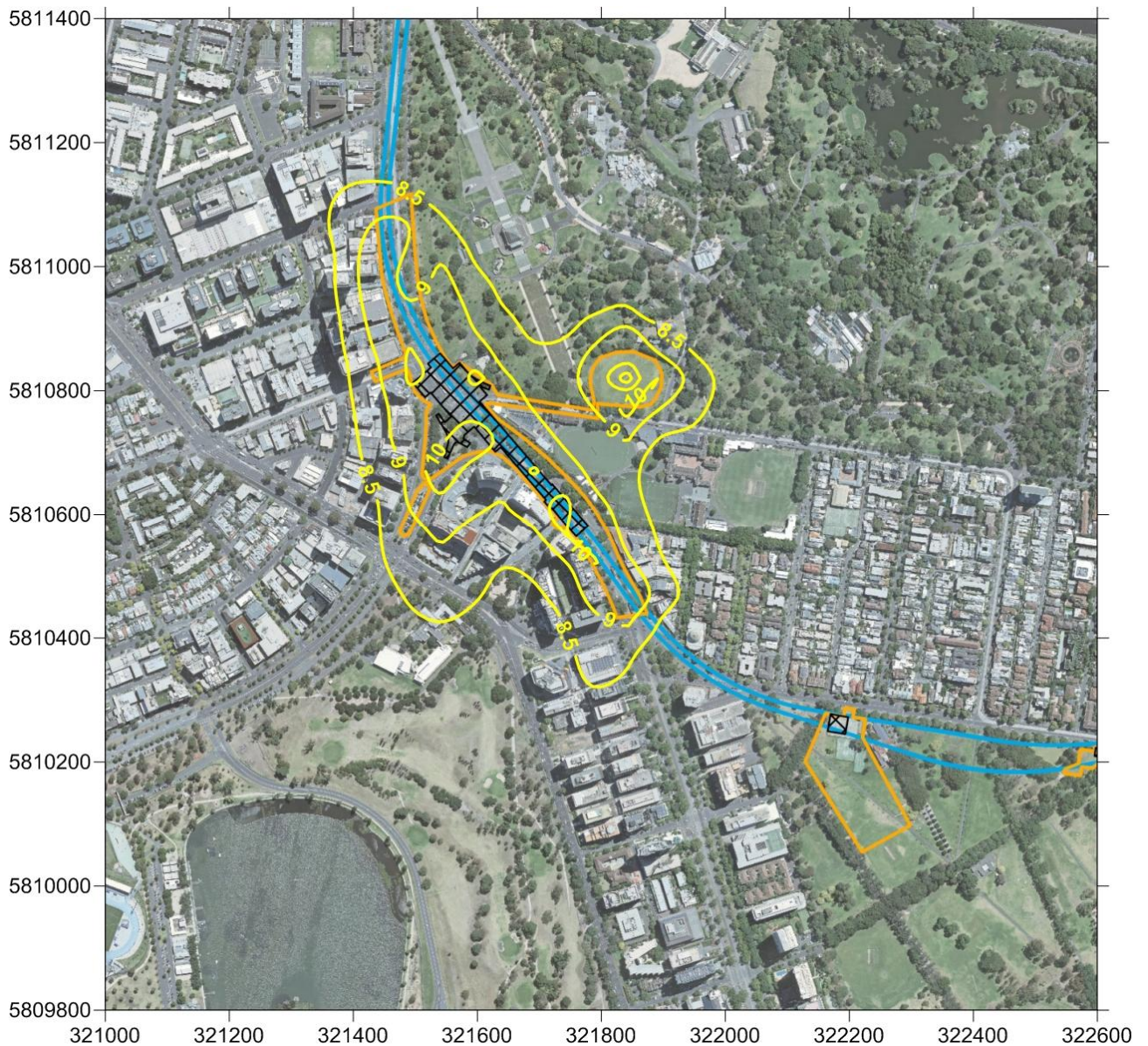
Figure 13-2 AERMOD results for maximum 24-hour average PM 2.5 GLC
