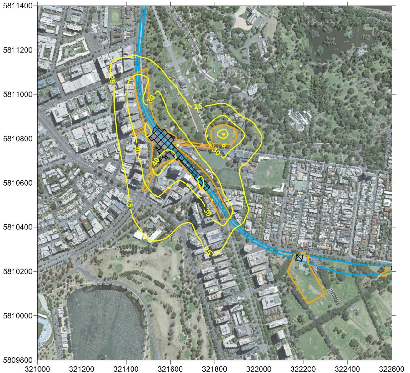
Figure 13-1 AERMOD results for maximum 24-hour average PM 10 GLC
