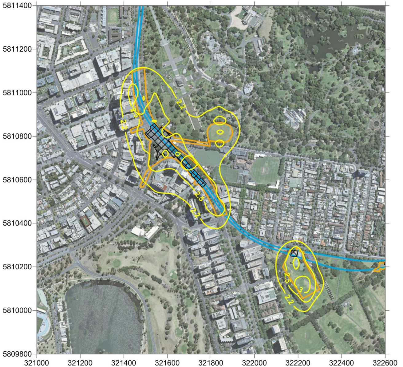
Figure 13-8 AERMOD results for monthly average dust deposition.
