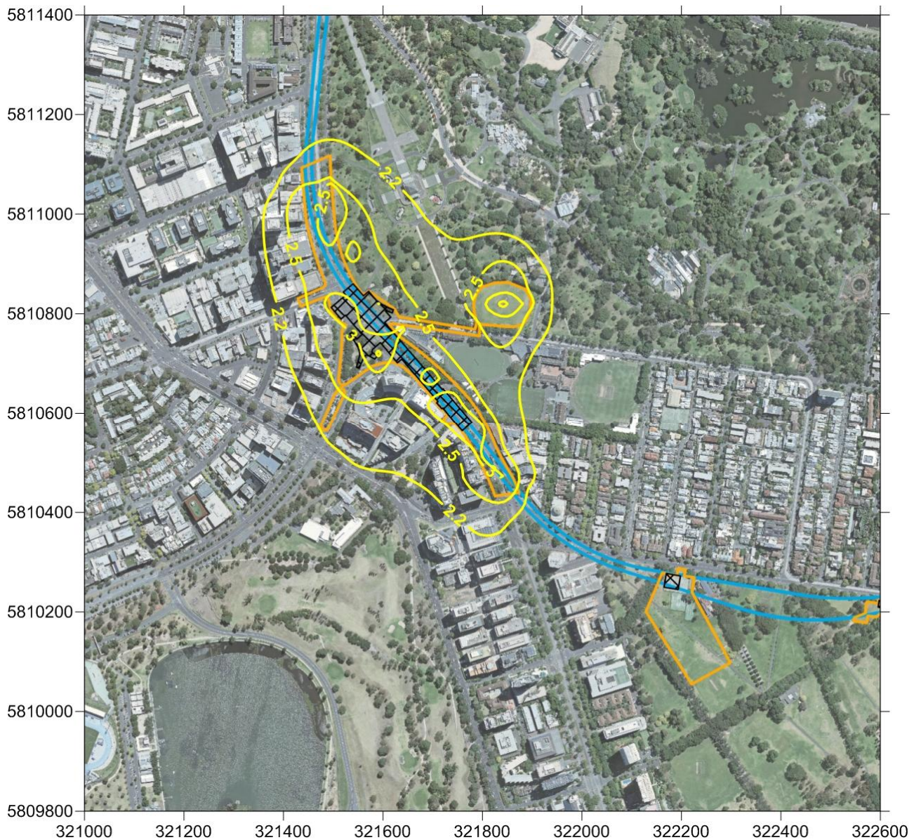
Figure 13-4 AERMOD results for monthly average dust deposition.
