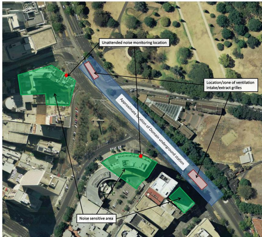
**Figure D.8: Location of fixed noise sources, measurements of attended background noise levels (red dots) and Noise Sensitive Areas**
