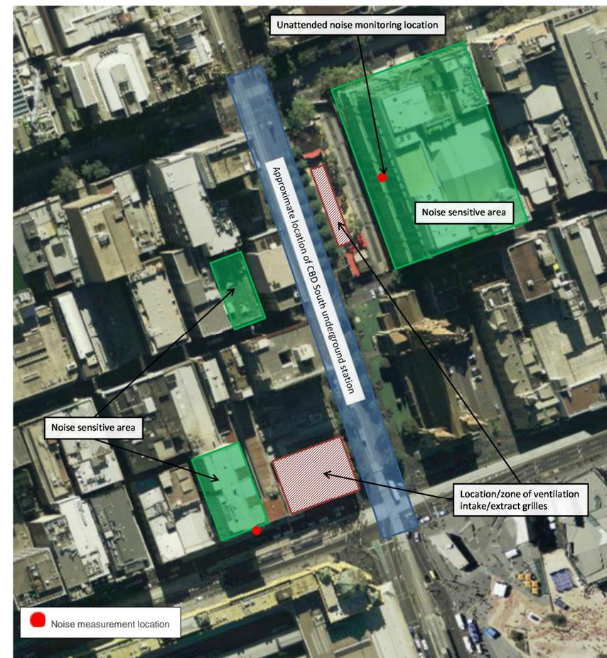
Figure D.7: Location of fixed noise sources, measurements of attended background noise levels (red dots) and Noise Sensitive Areas for Precinct 6
