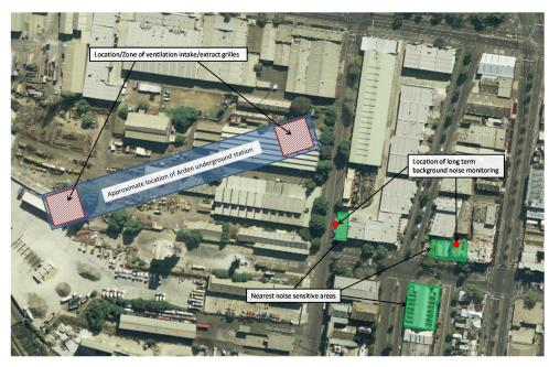
Figure D.4: Location of fixed noise sources, measurements of background noise levels and Noise Sensitive Areas for Precinct 3
