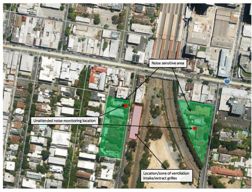
Figure D.9: Location of fixed noise sources, measurements of attended background noise levels (red dots) and NSAs
