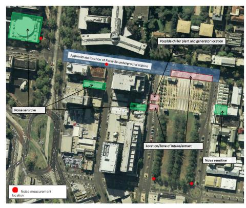
Figure D.5: Location of fixed noise sources, measurements of attended background noise levels (red dots) and Noise Sensitive Areas for Precinct 4
