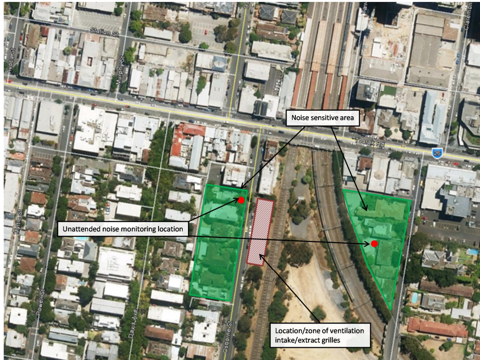
Figure D.9: Location of fixed noise sources, measurements of attended background noise levels (red dots) and NSAs
