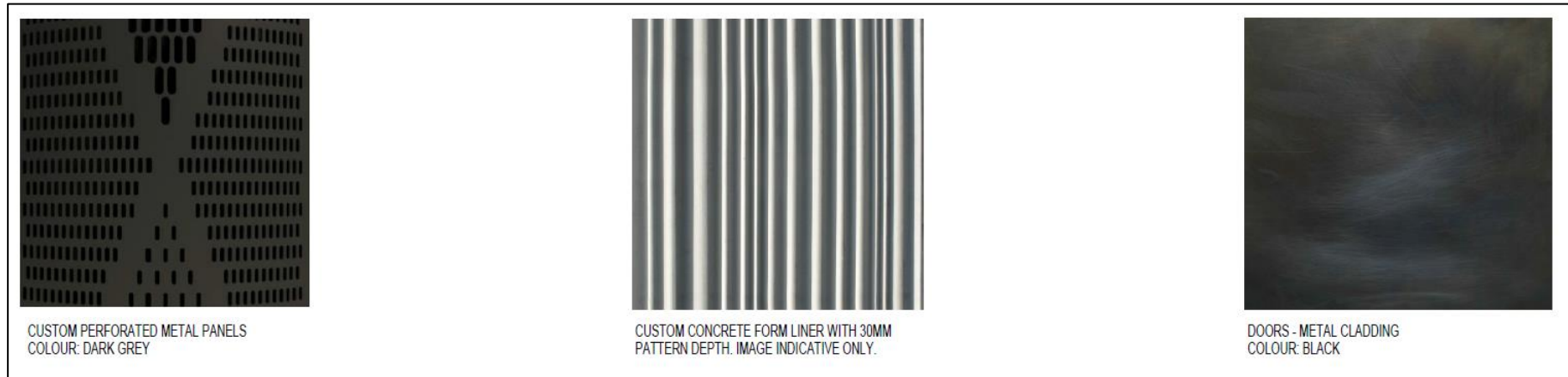
Figure 8 – Materials and finishes at the Western Portal
