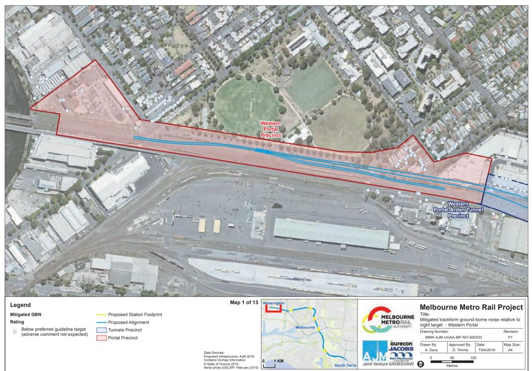
Figure E.36: Mitigated Ground-borne Noise Levels due to Trains in Precinct 2: Western Portal
