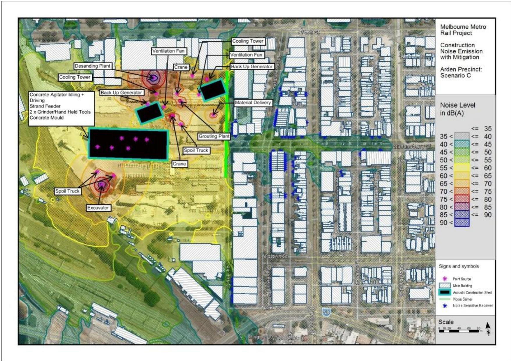
Figure A.57: Arden Precinct Scenario C Predicted Noise Levels at 1.5 m above ground – construction activities to be undertaken over 24 hours Unavoidable Works – with additional mitigation
