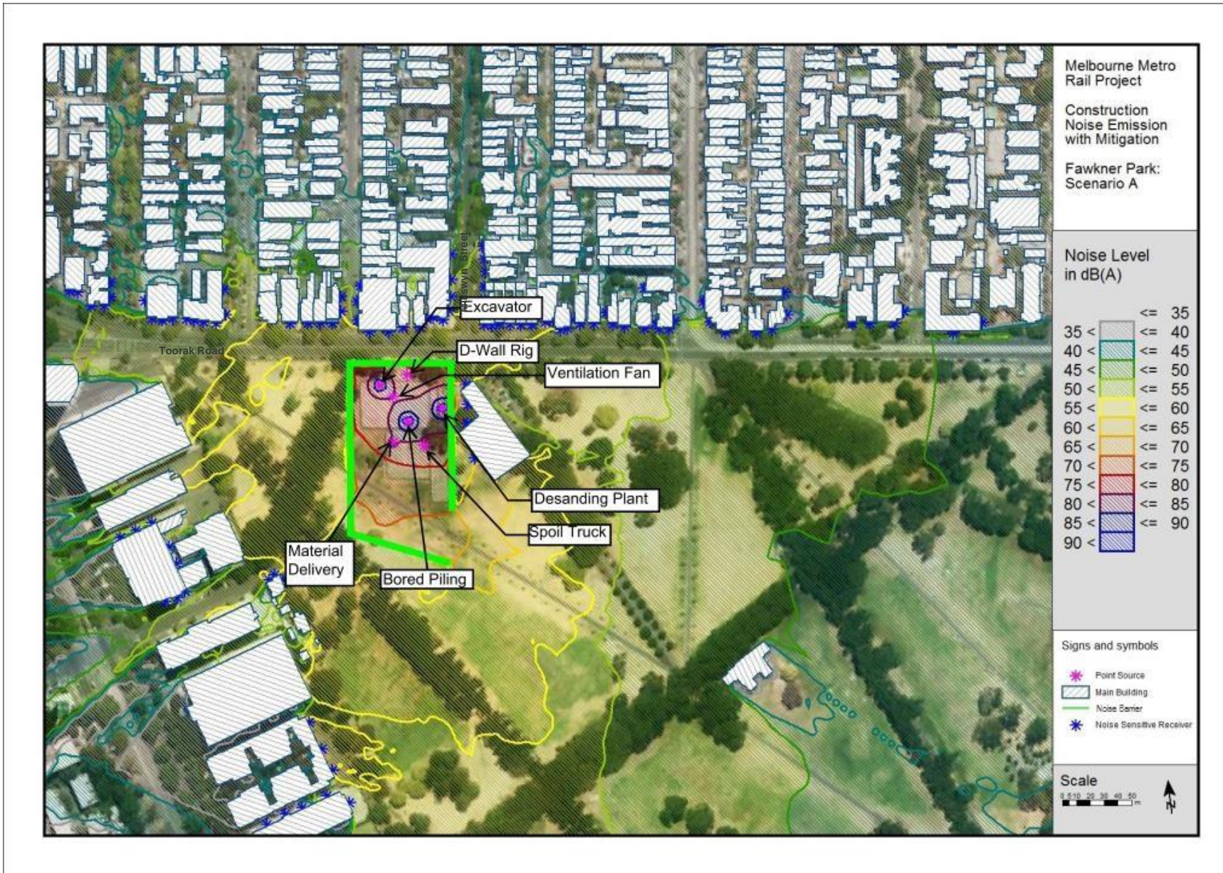
Figure A.44: Tunnels Precinct Fawkner Park Scenario A Predicted Noise Levels at 1.5 m above ground – construction activities to be undertaken during Normal Working Hours – with additional mitigation
