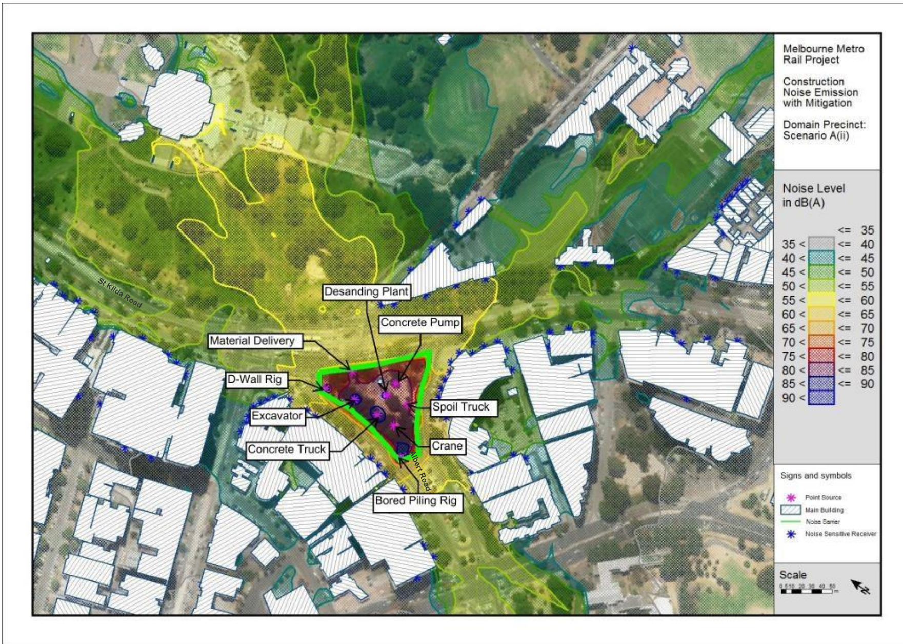
Figure A.64: Domain Precinct Scenario A(ii) Predicted Noise Levels at 1.5 m above ground – construction activities to be undertaken during Normal Working Hours – with additional mitigation
