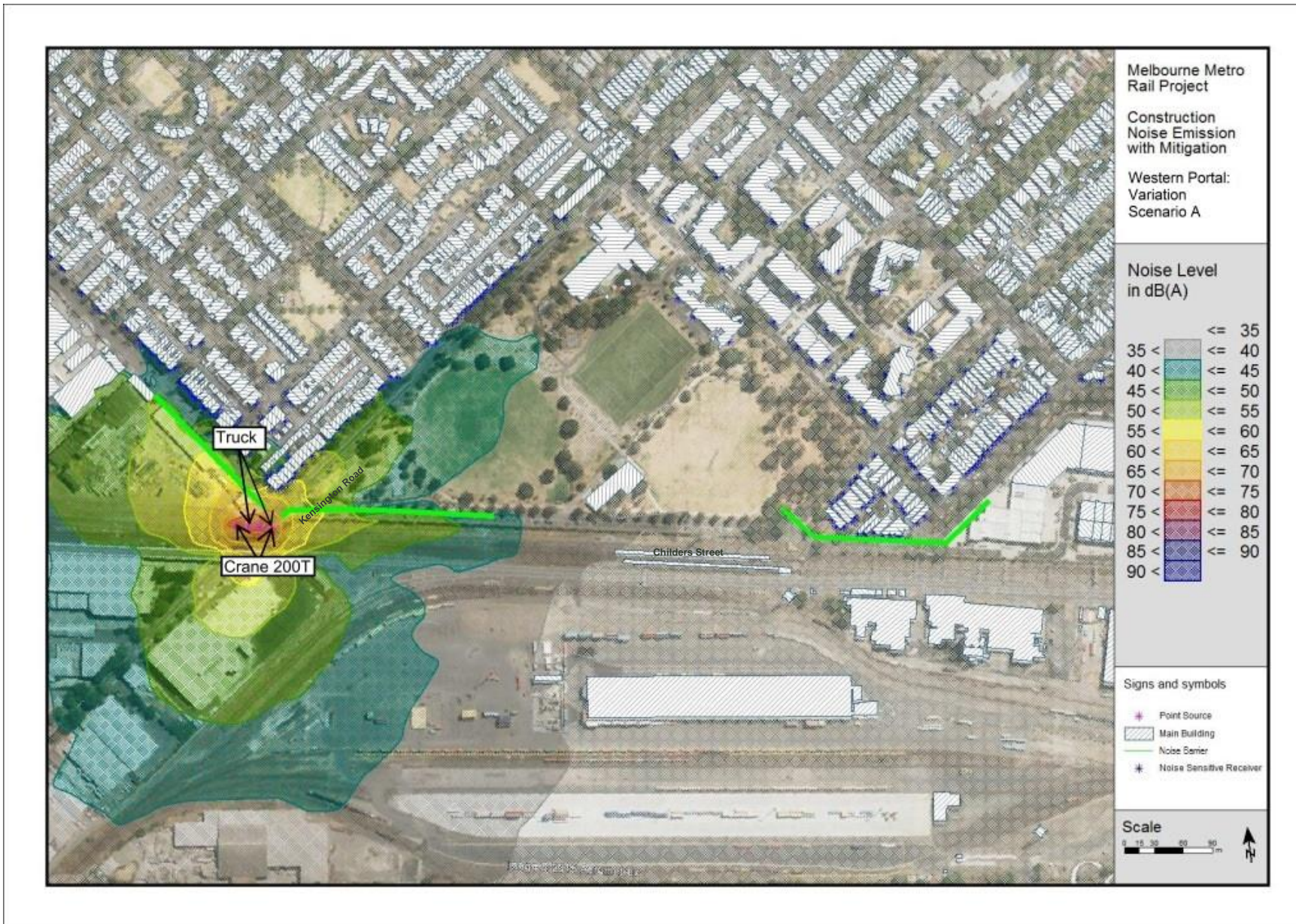
Figure A.51: Western Portal Construction Alternative Design Options, Scenario A Predicted Noise Levels at 1.5 m above ground – construction activities to be undertaken over 24 hours Unavoidable Work – with additional mitigation
