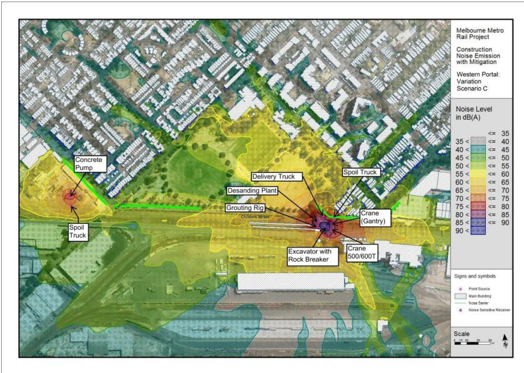
Figure A.53: Western Portal Construction Alternative Design Options, Scenario C Predicted Noise Levels at 1.5 m above ground – construction activities to be undertaken during Normal Working Hours – with additional mitigation
