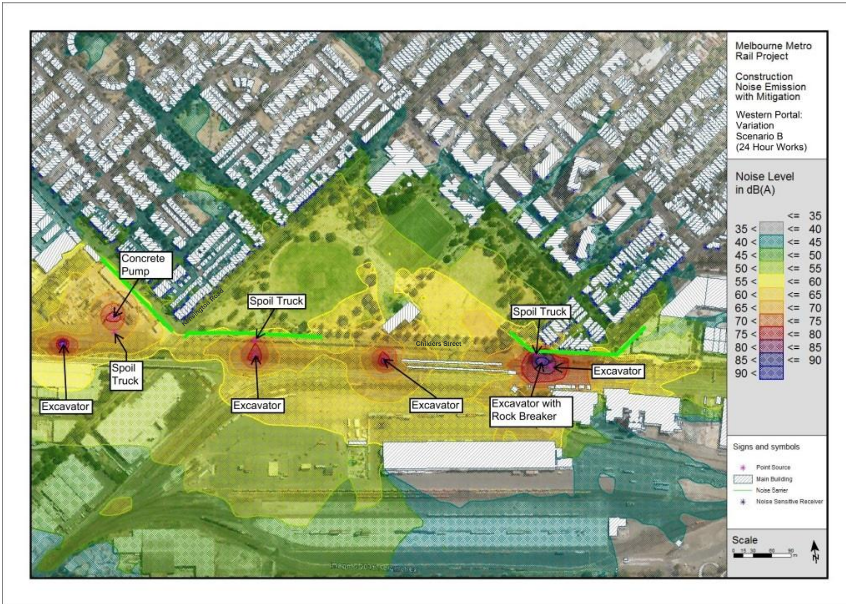
Figure A.52: Western Portal Construction Alternative Design Options, Scenario B Predicted Noise Levels at 1.5 m above ground – construction activities to be undertaken over 24 hours Unavoidable Work – with additional mitigation
