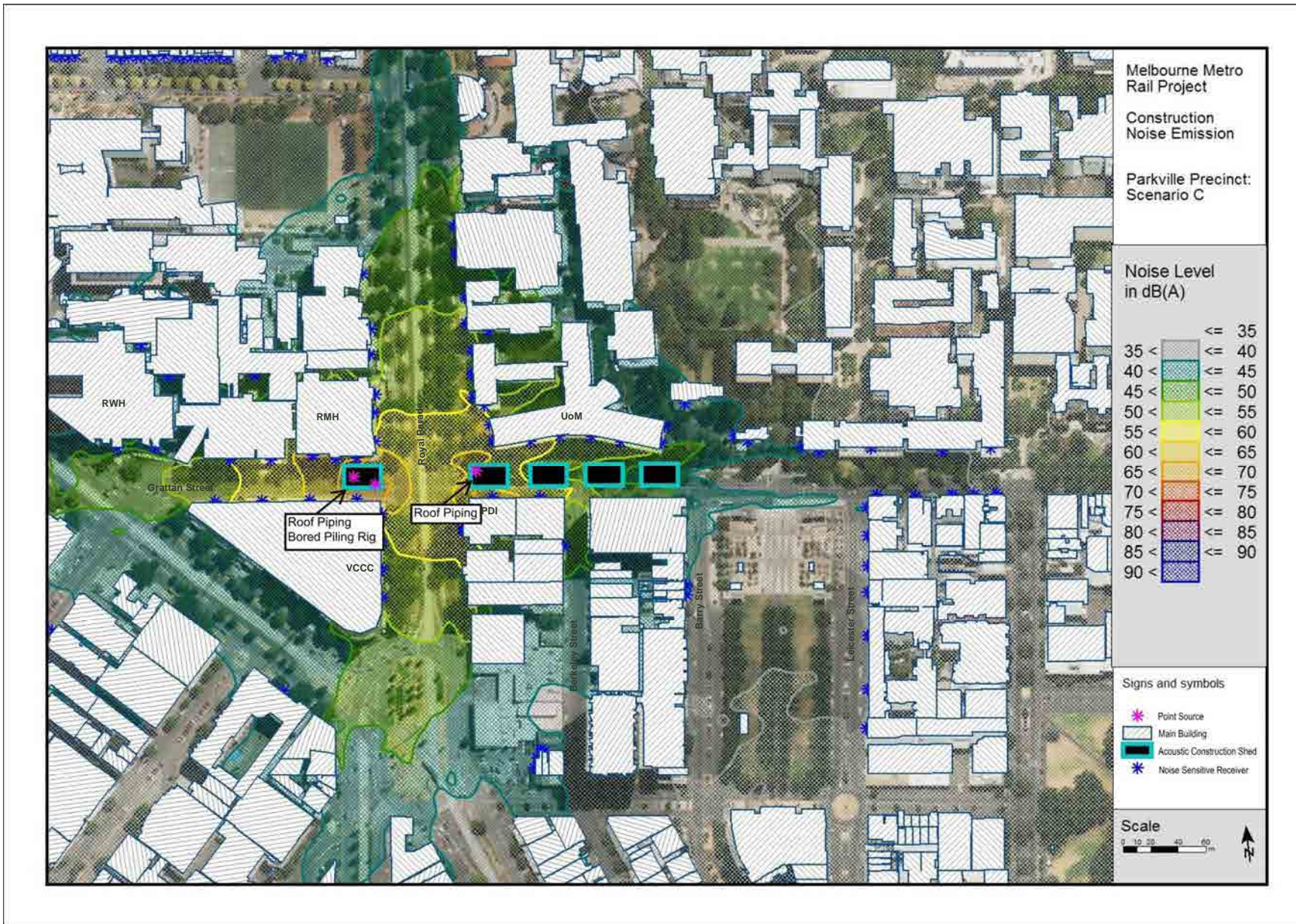
Figure A.21: Parkville Station Precinct - Scenario C - Predicted Noise Levels at 1.5 m above ground - Construction activities to be undertaken during Normal Working Hours
