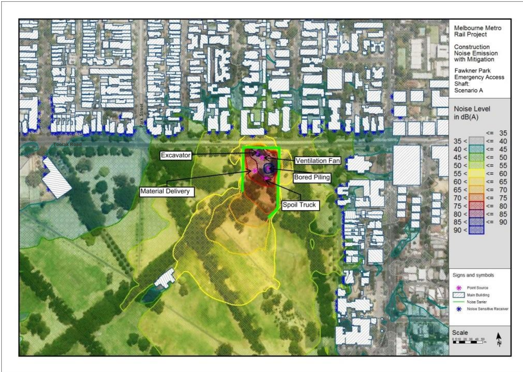
Figure A.47: Fawkner Park Emergency Access Shaft Scenario A Predicted Noise Levels at 1.5 m above ground – construction activities to be undertaken during Normal Working Hours – with additional mitigation
