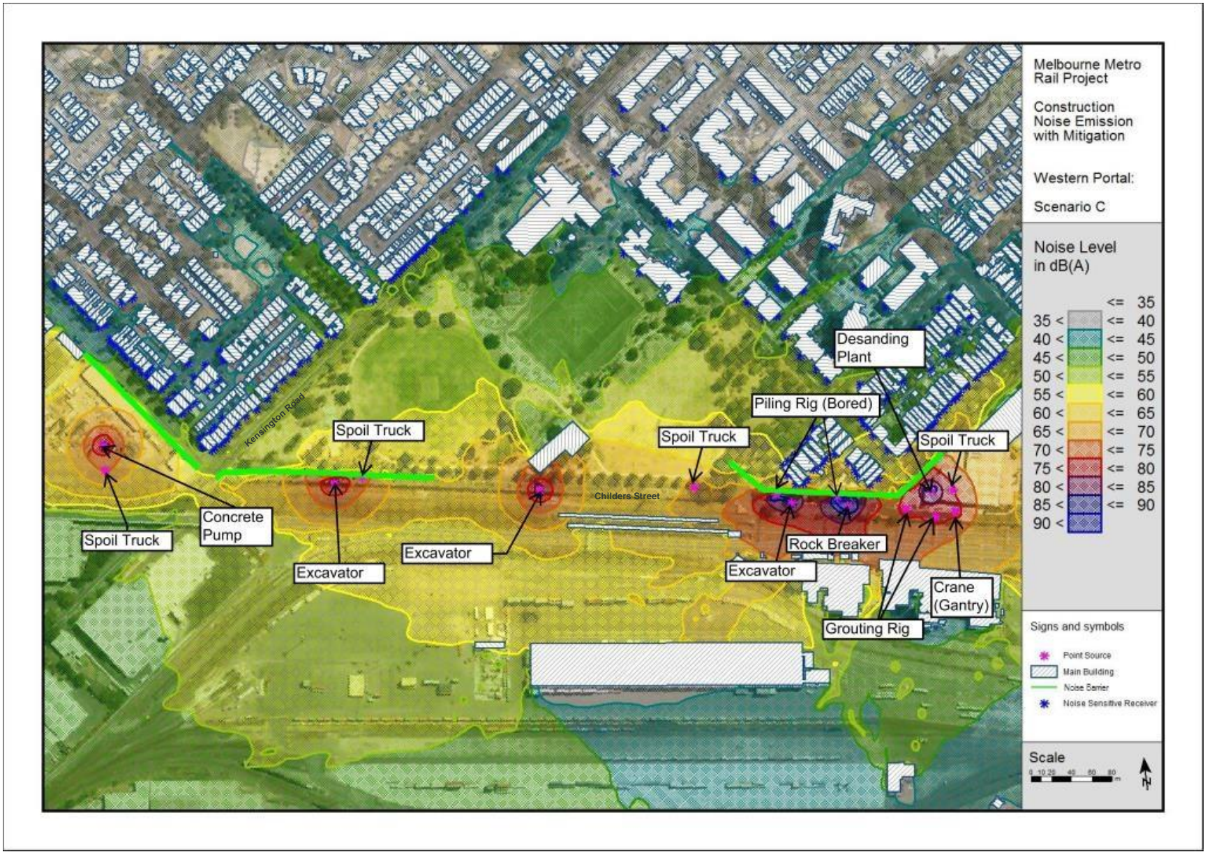
Figure A.50: Western Portal Construction Design, Scenario C Predicted Noise Levels at 1.5 m above ground – construction activities to be undertaken during Normal Working Hours – with additional mitigation
