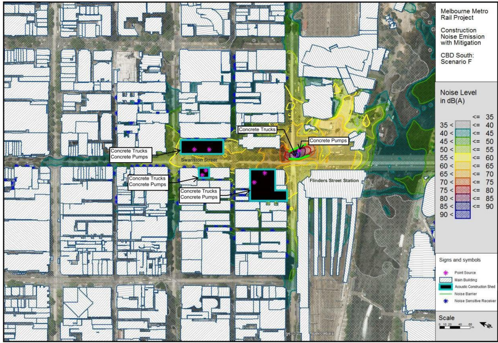
Figure A.62: CBD South Precinct Scenario F Predicted Noise Levels at 1.5 m above ground – construction activities to be undertaken over 24 hours Unavoidable Work – with additional mitigation
