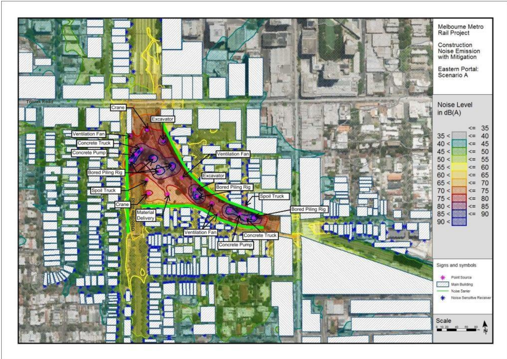
Figure A.65: Eastern Portal Precinct Scenario A Predicted Noise Levels at 1.5 m above ground – construction activities to be undertaken over 24 hours Unavoidable Work – with additional mitigation
