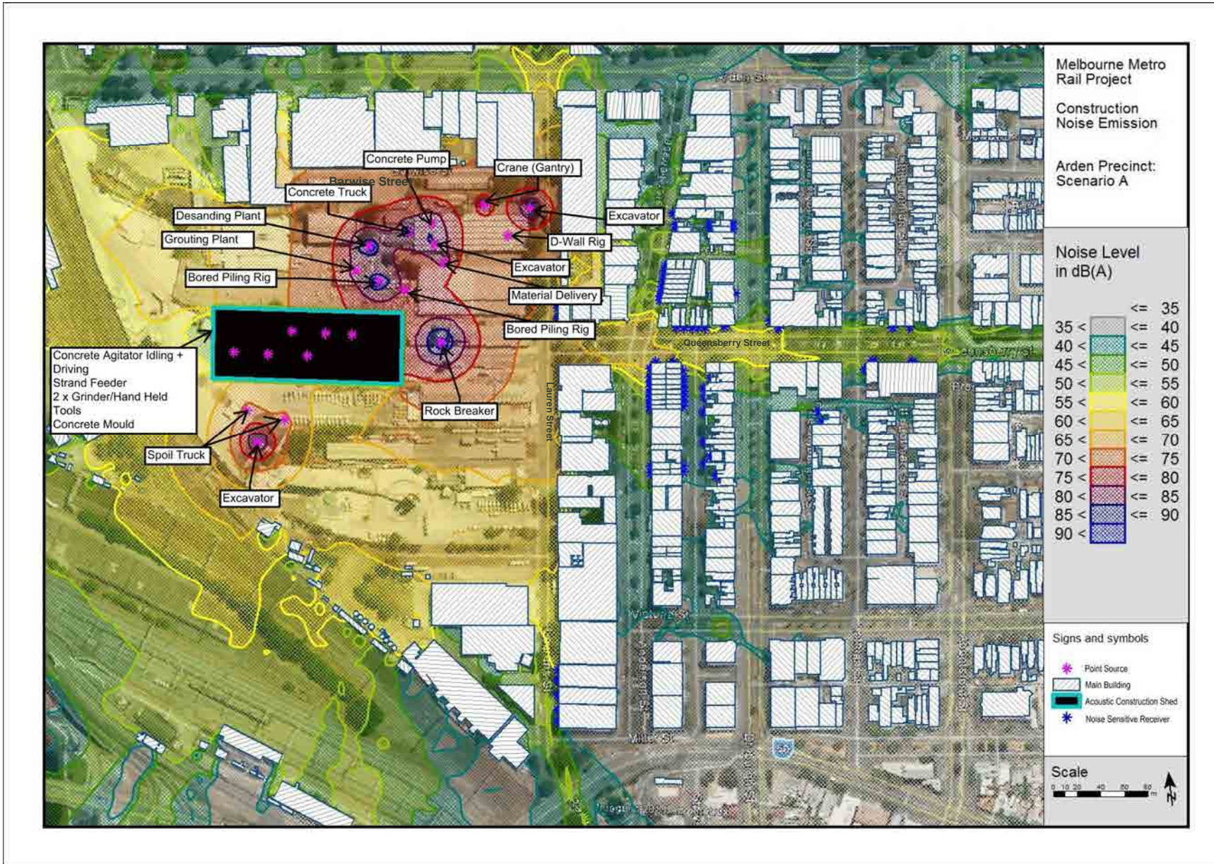
Figure A.15: Arden Station Precinct Scenario A - Predicted Noise Levels at 1.5 m above ground - construction activities to be undertaken over Normal Working Hours
