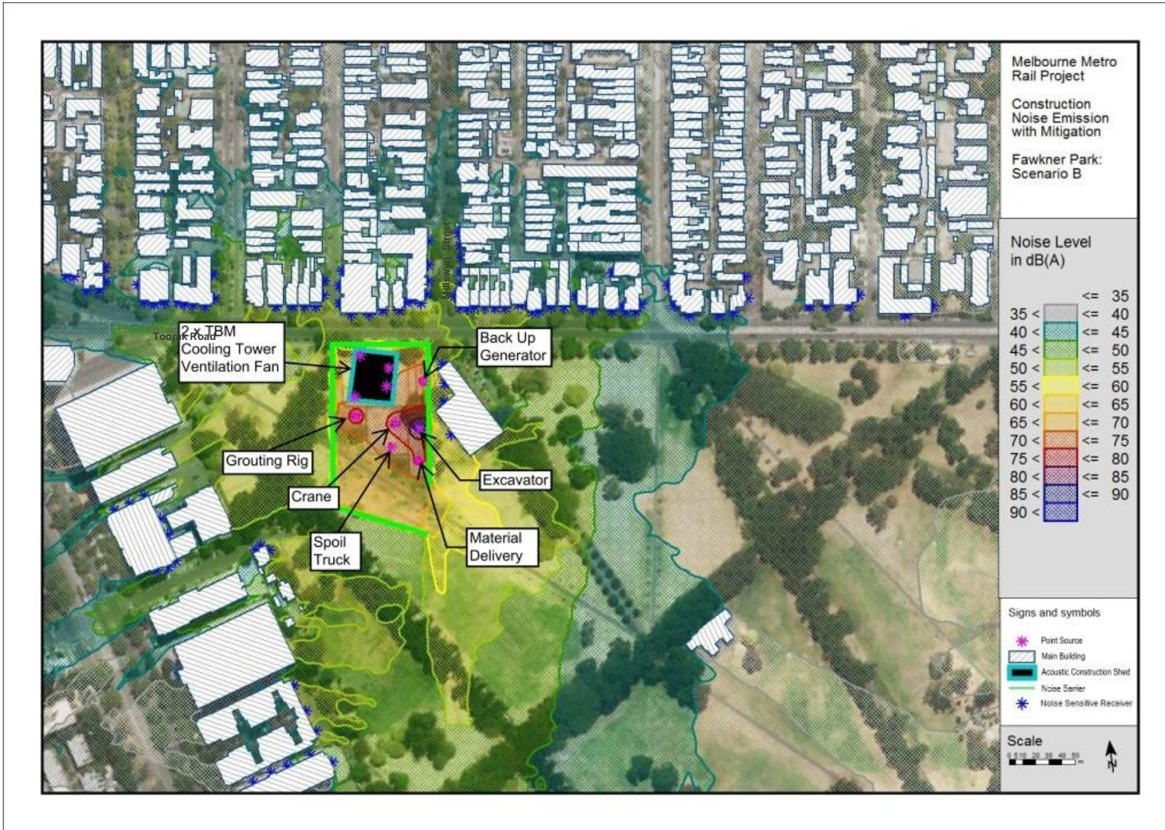
Figure A.45: Tunnels Precinct Fawkner Park Scenario B Predicted Noise Levels at 1.5 m above ground – construction activities to be undertaken over 24-hours Hours Unavoidable Works – with additional mitigation
