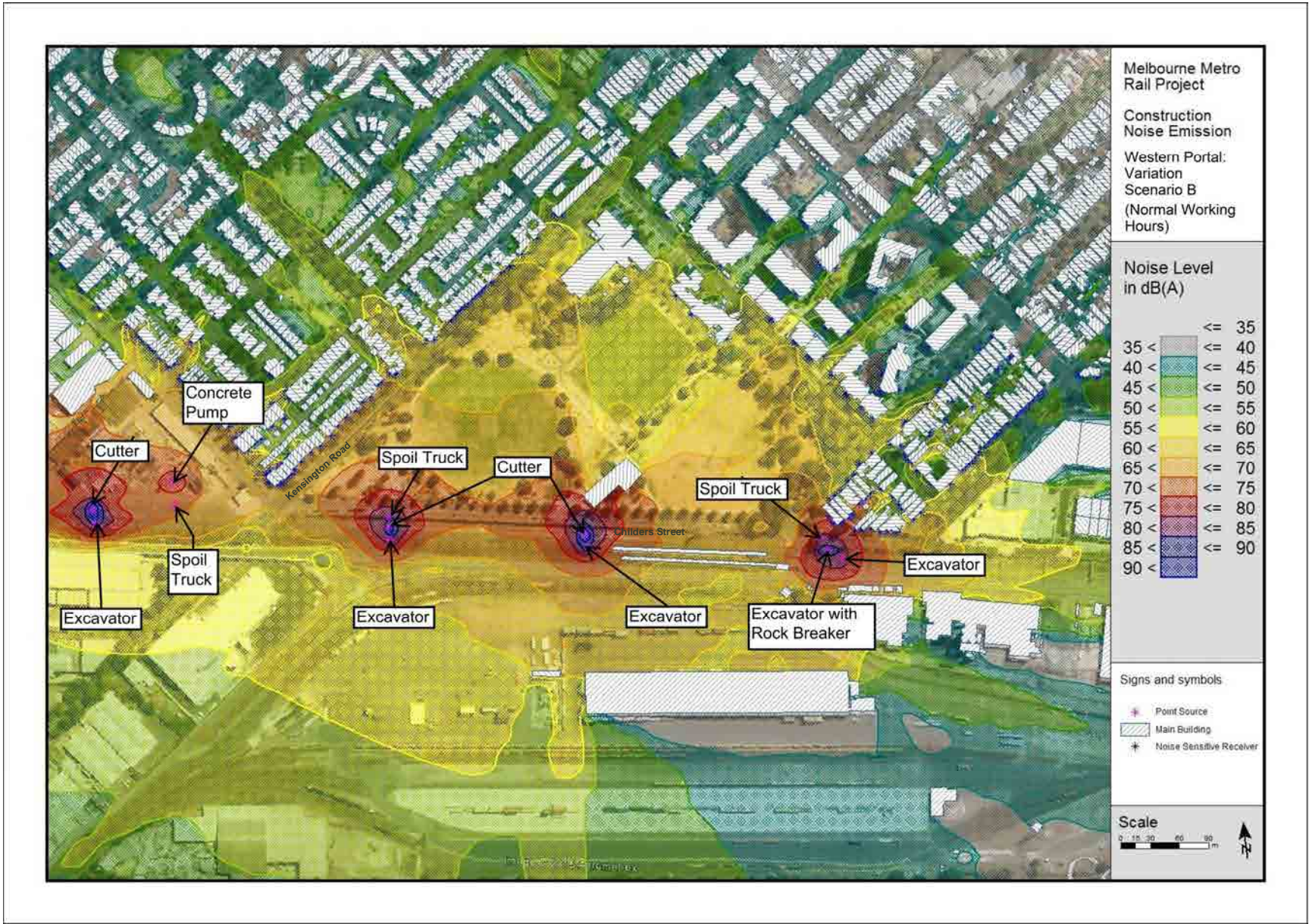
Figure A.12: Western Portal Construction - Alternative Design Options, Scenario B(ii) - Predicted Noise Levels at 1.5 m above ground - construction activities to be undertaken during Normal Working Hours to allow for rail cutting activities
