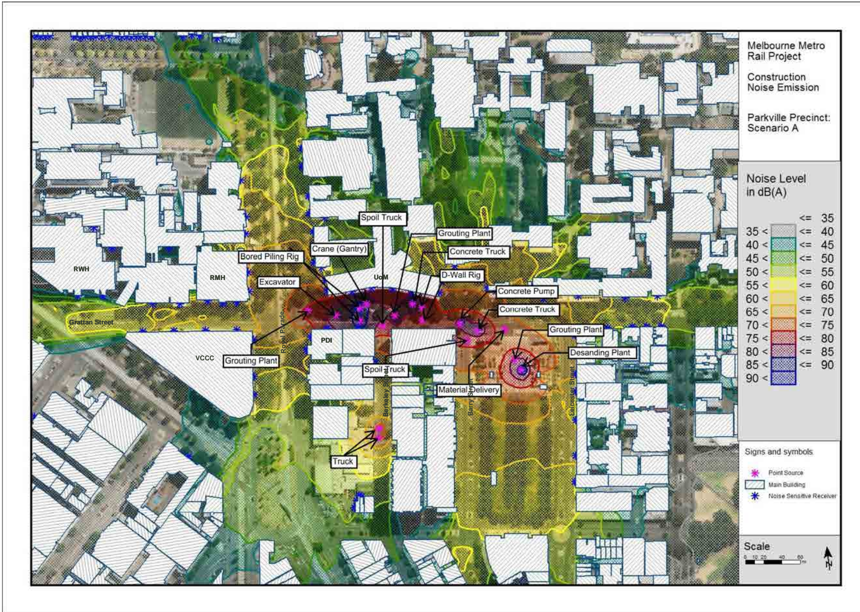
Figure A.19 : Parkville Station Precinct - Scenario A - Predicted Noise Levels at 1.5 m above ground - Construction activities to be undertaken during Normal Working Hours
