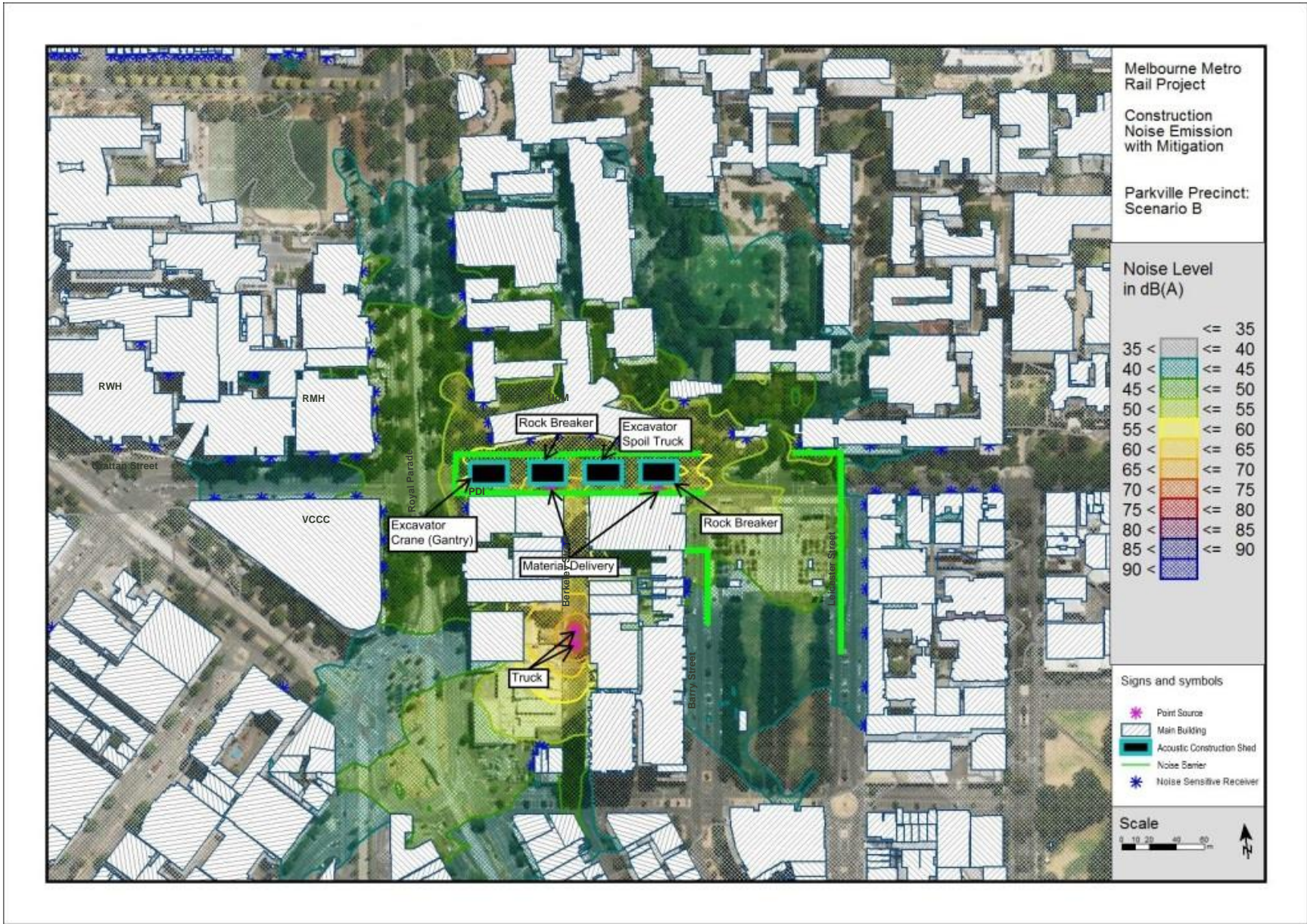
Figure A.60: Parkville Precinct Scenario B Predicted Noise Levels at 1.5 m above ground – construction activities to be undertaken over 24 hours – with additional mitigation
