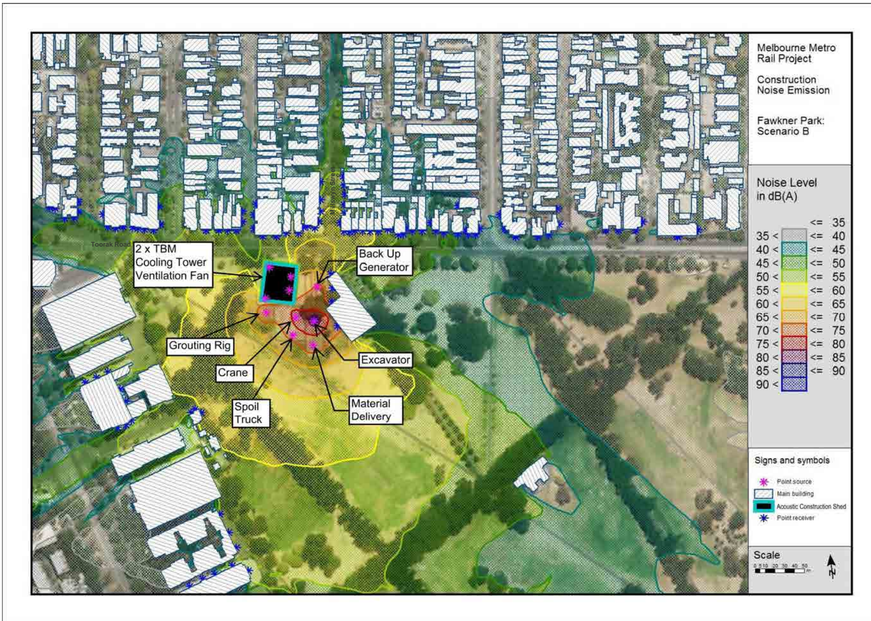
Figure A.2: Fawcner Park Construction Scenario B - Predicted Noise Levels at 1.5 m above ground - construction activities to be undertaken over 24 hours Unavoidable Works
