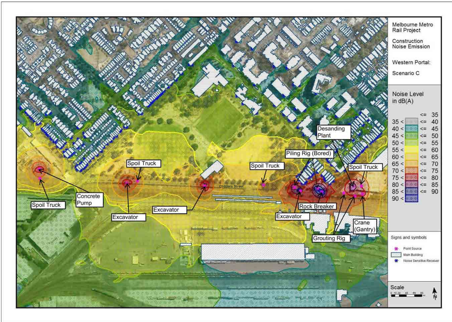
Figure A.9: Western Portal Construction - Design, Scenario C - Predicted Noise Levels at 1.5 m above ground - construction activities to be undertaken during Normal Working Hours
