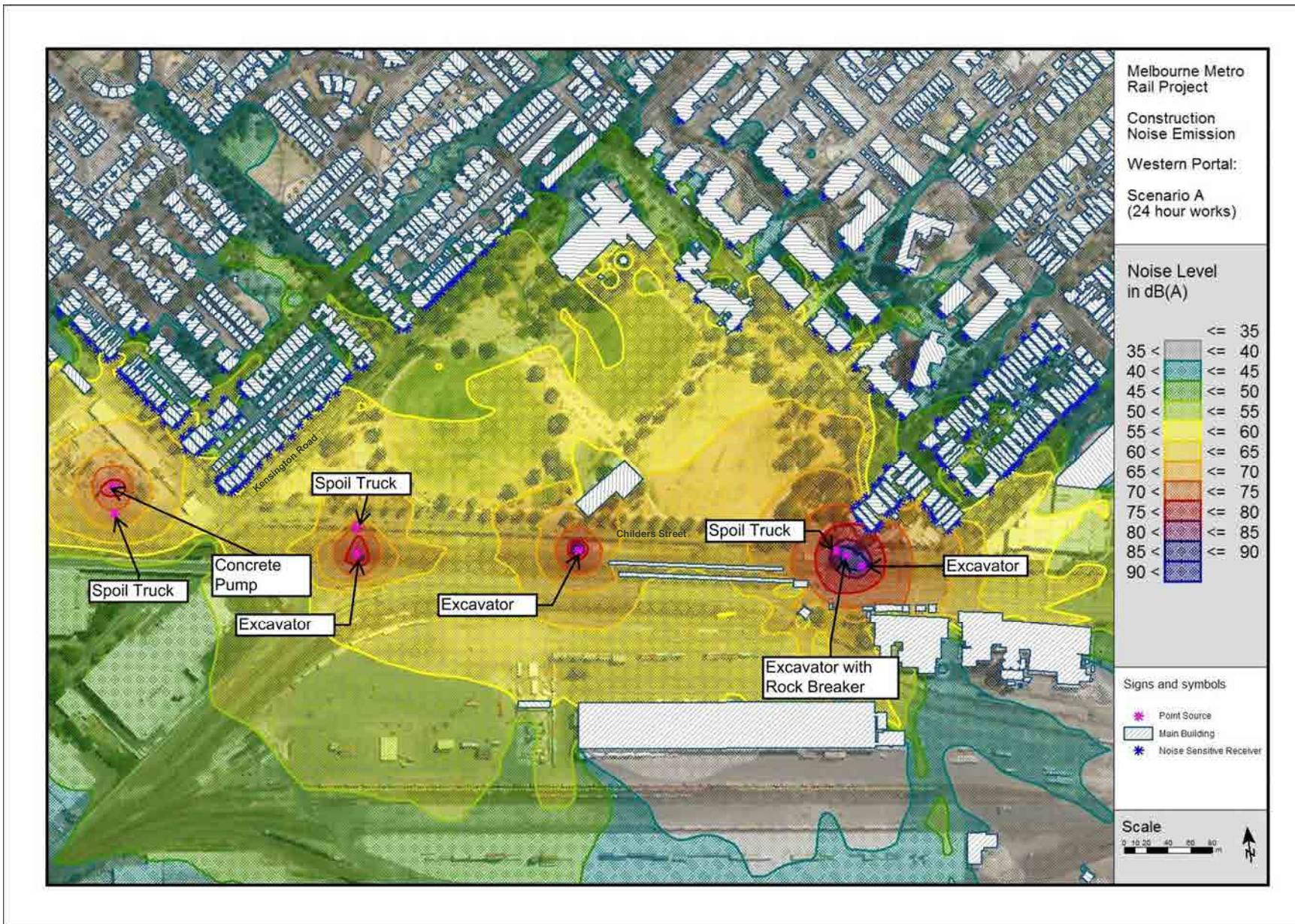
Figure A.6: Western Portal Construction – Design, Scenario A(i) - Predicted Noise Levels at 1.5 m above ground - construction activities to be undertaken over 24 hours Unavoidable Works
