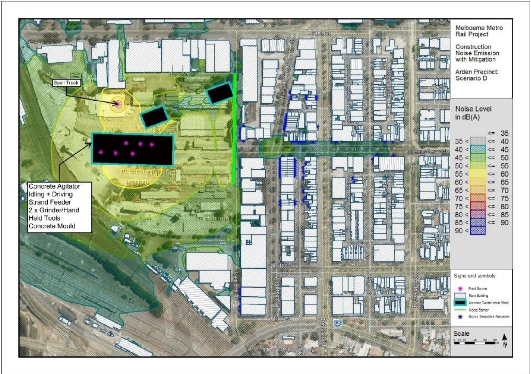
Figure A.58: Arden Precinct Scenario D Predicted Noise Levels at 1.5 m above ground – construction activities to be undertaken over 24 hours – with additional mitigation
