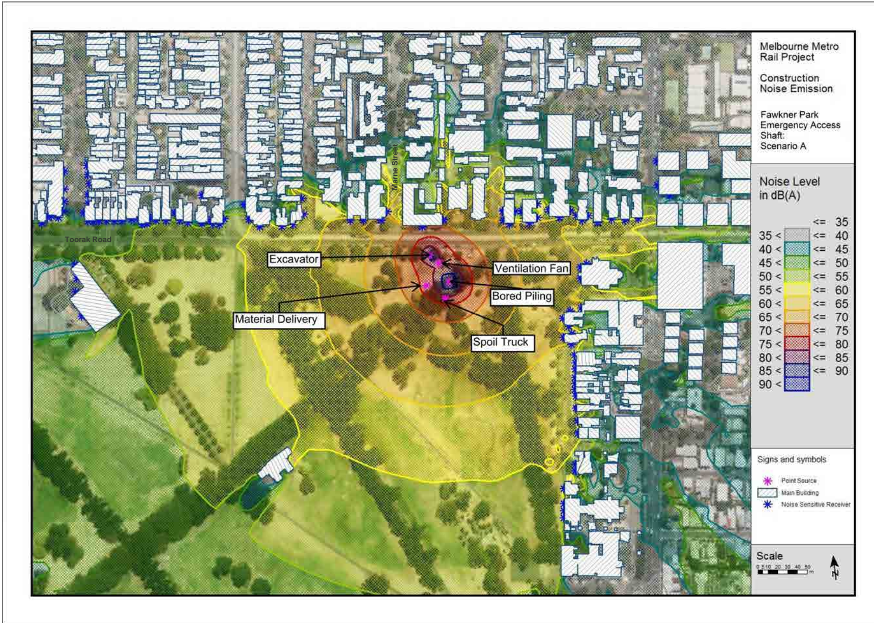
Figure A.5: Fawkner Park Emergency Access Shaft Construction Scenario A - Predicted Noise Levels at 1.5 m above ground - construction activities to be undertaken during Normal Working Hours
