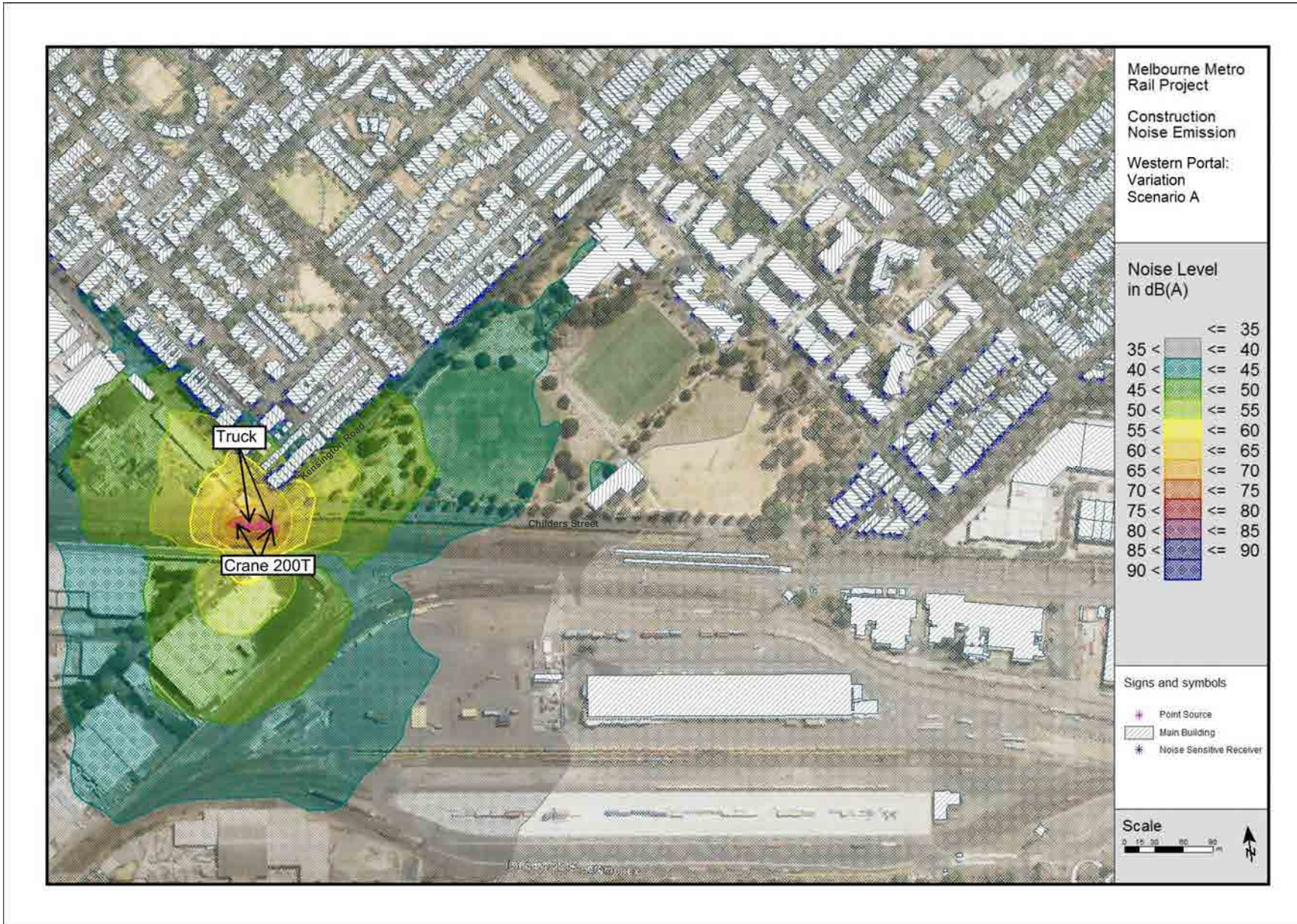
Figure A.10: Western Portal Construction - Alternative Design Options, Scenario A - Predicted Noise Levels at 1.5 m above ground - construction activities to be undertaken over 24 hours Unavoidable Works
