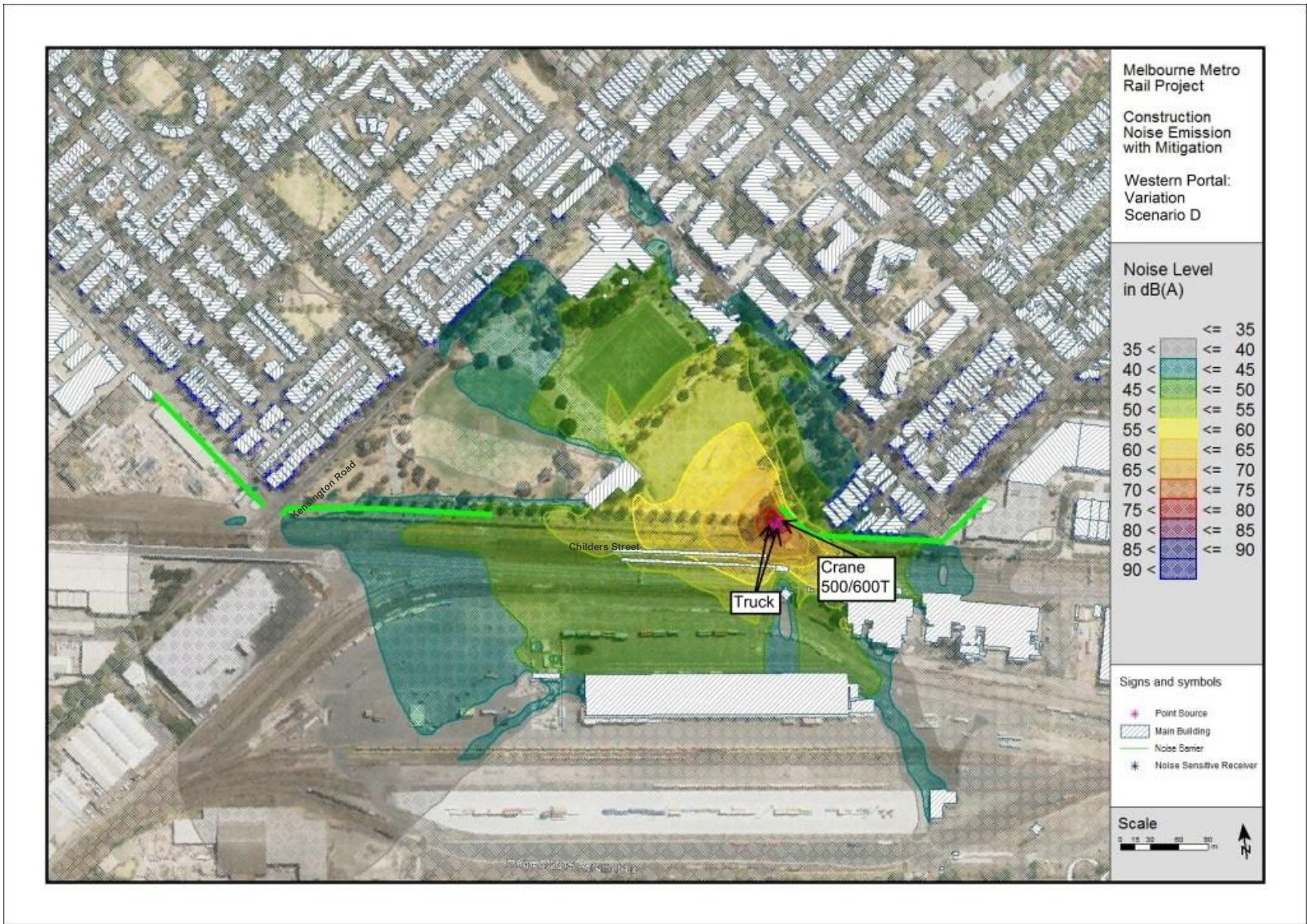
Figure A.54: Western Portal Construction Alternative Design Options, Scenario D Predicted Noise Levels at 1.5 m above ground – construction activities to be undertaken over 24 hours Unavoidable Work – with additional mitigation
