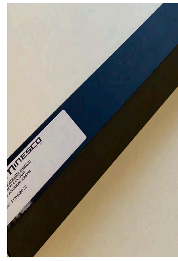
Service core - black aluminium anodised louvers + frames - Little LaTrobe East & West
