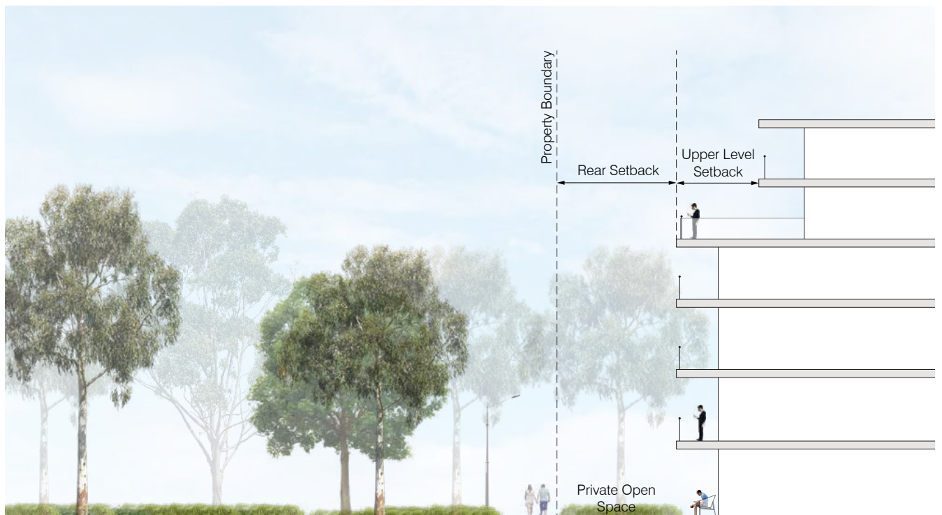
Figure 35: Section D - Indicative cross section along the eastern interface of Surrey Park.
