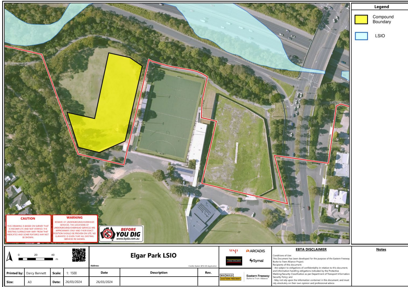
Figure 7: 100-year ARI Flood Zone (LSIO)
