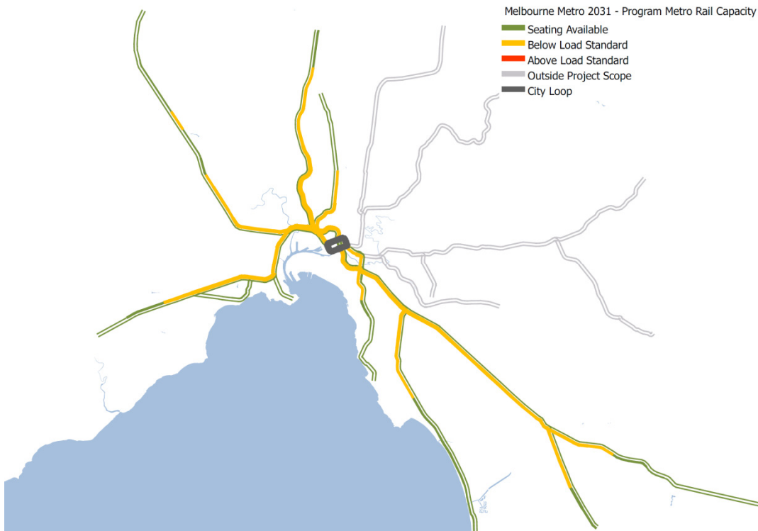
Figure 20: Crowding on the train network in 2031 with Melbourne Metro Program (volume/capacity ratio)
