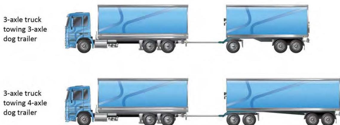
Figure 10-2 – Example truck and dog combinations
