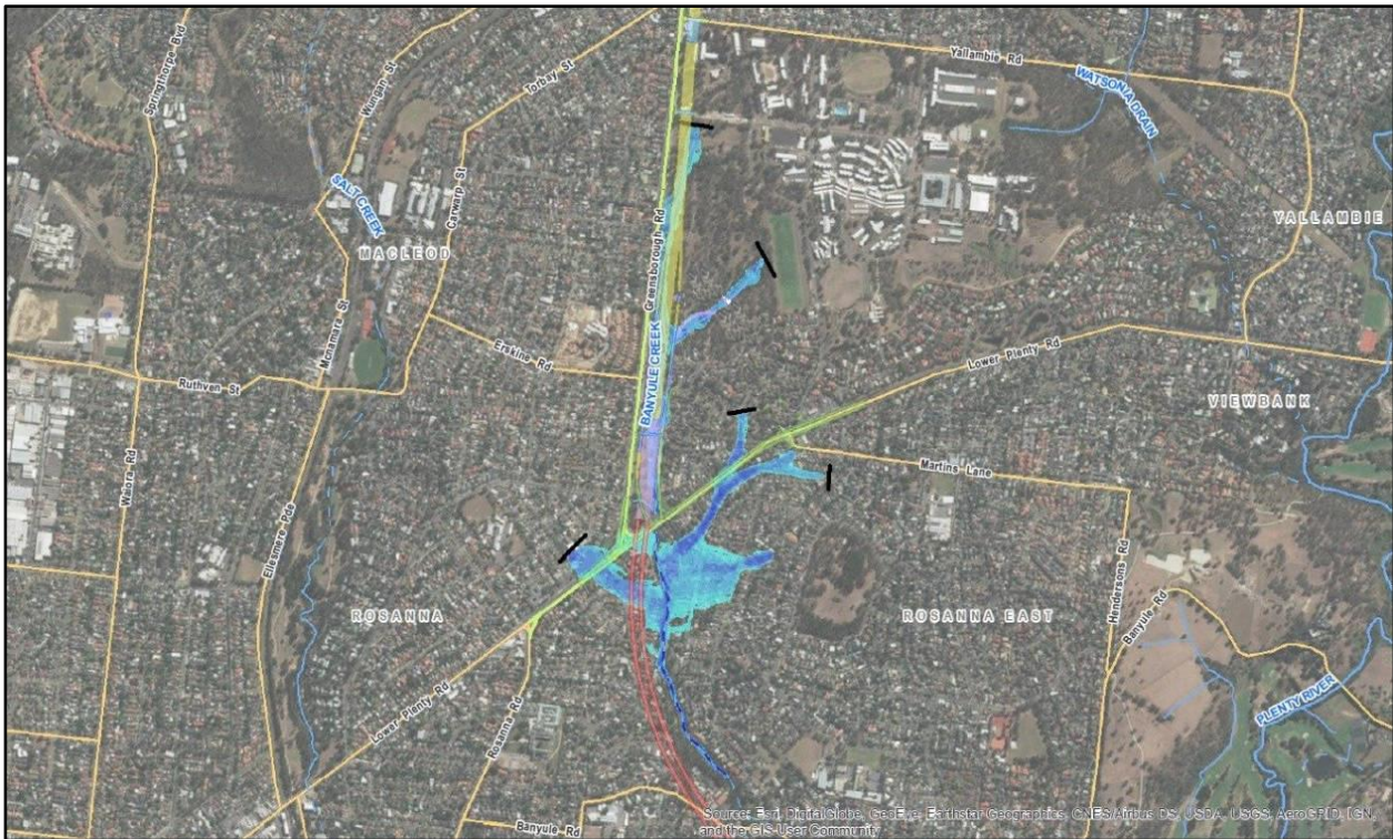
Figure 22 Banyule Creek 1% AEP existing conditions maximum flood depths
