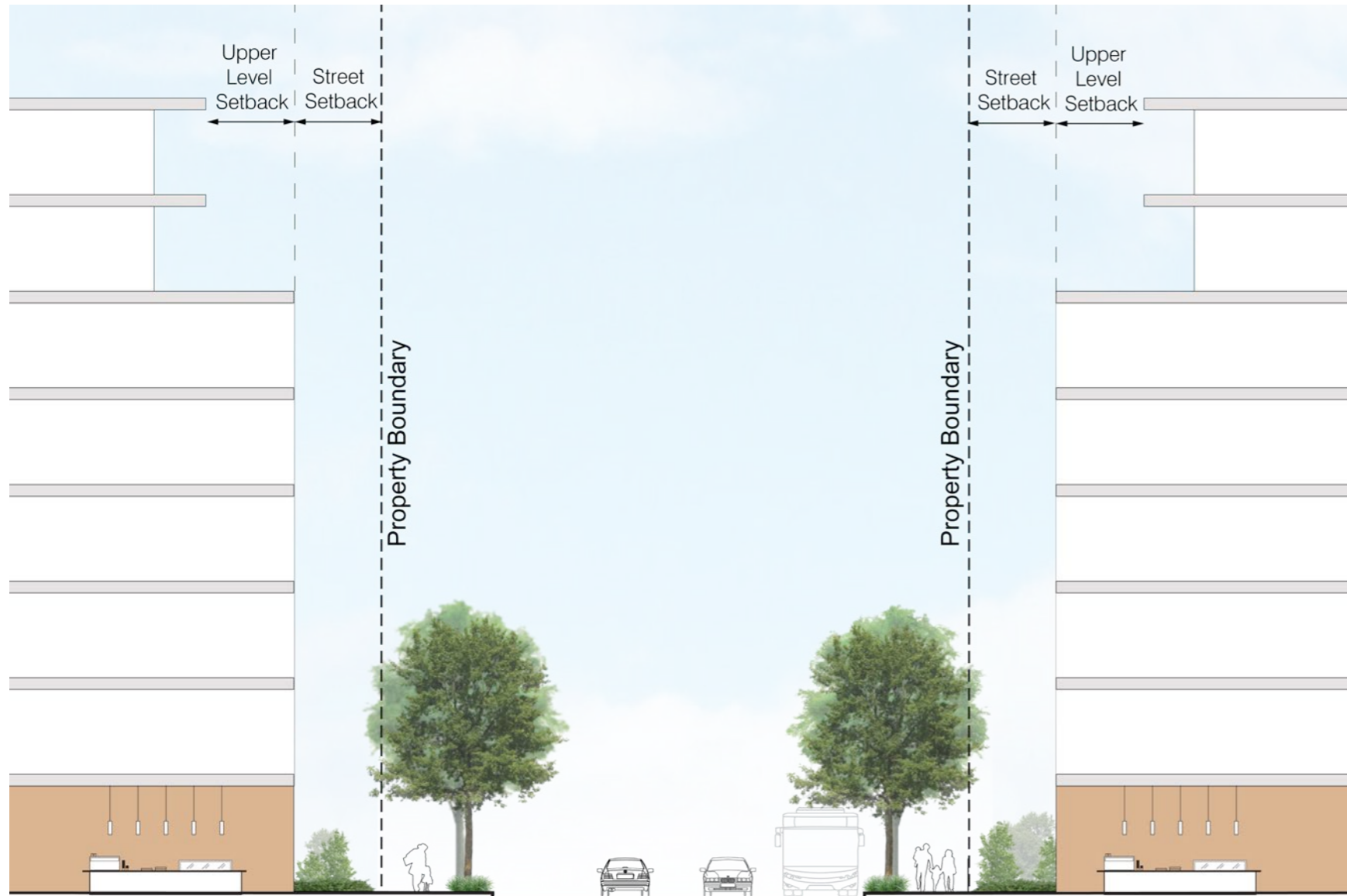
Figure 6.22: Potential section - Avenue
