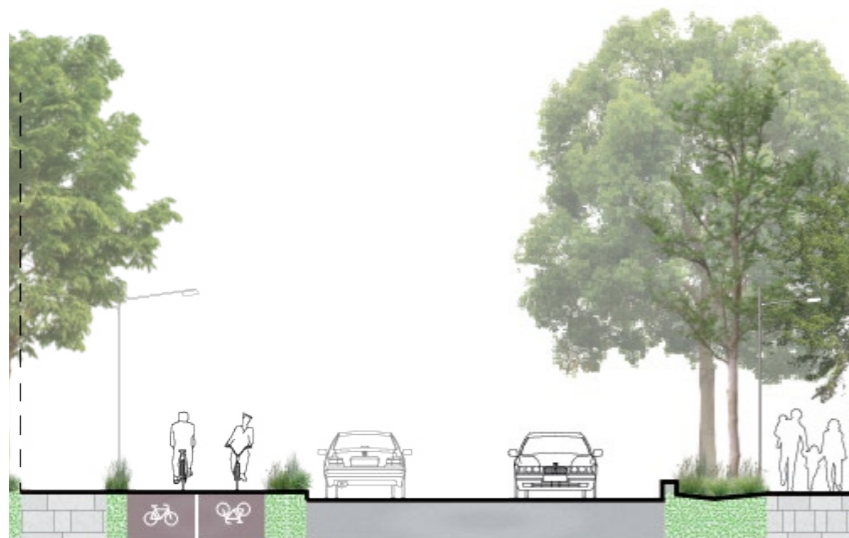
Figure 3.12: Indicative section, Green Street - Type C - Cycling
