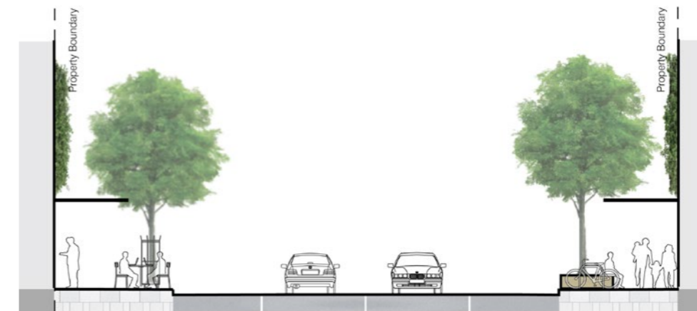
Figure 3.10: Indicative section, Activity Street - Type A
